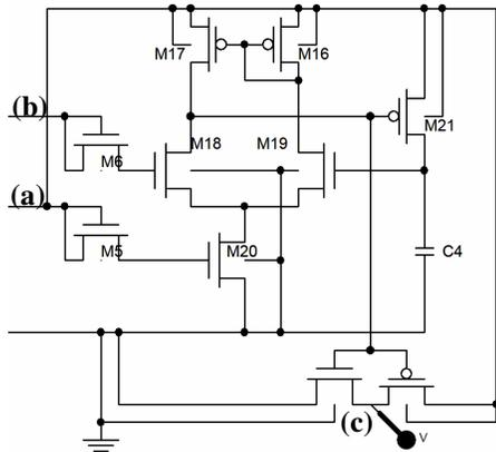
Figure 6 – Peak detector circuit: (a) VDD, (b) full wave rectified, and (c) charge control output
