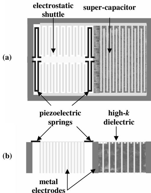
**Figure 1** – Concept drawing of HALF-LIVES system:
