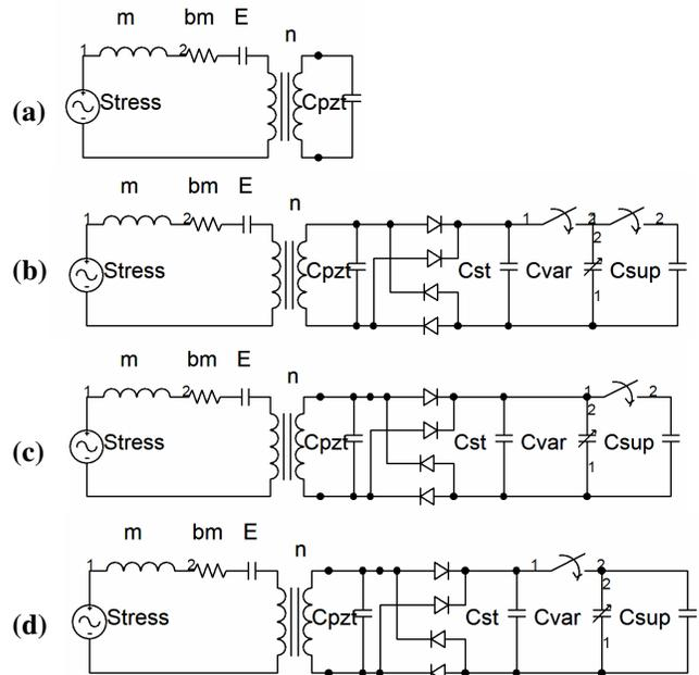
Figure 3 – Stages of scavenging operation: (a) piezoelectric elements disconnected, (b) full-wave rectified voltage charging temporary storage capacitor, (c) charge transfer to variable capacitor at  $C_{max}$ , (d) charge transfer from variable capacitor to supercapacitor at  $C_{min}$
