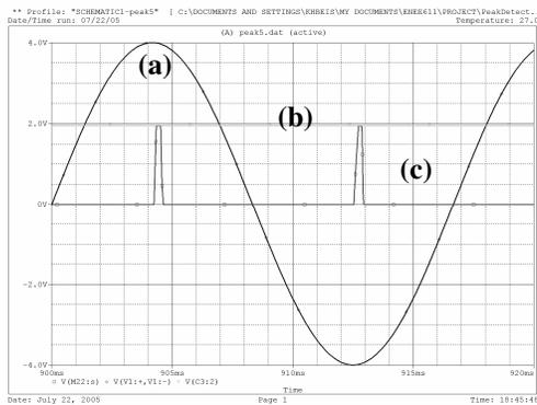
Figure 7 – PSpice simulation: (a) piezoelectric input voltage, (b) VDD, and (c) charge control signal
