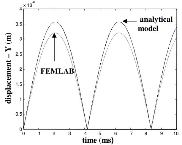
**Figure 4** – Comparison of FEMLAB simulation to analytical model for displacement in primary (Y) axis.
