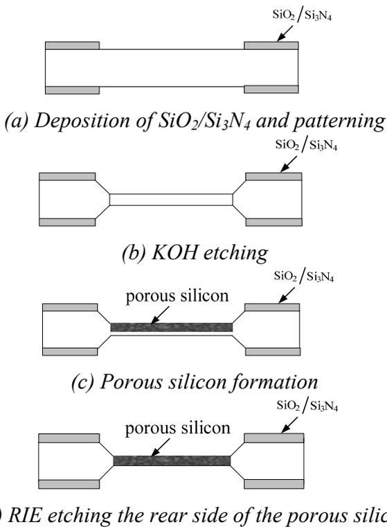
Fig. 2: Fabrication process of the porous silicon membranes.
