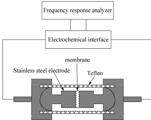
Fig. 5: Schematic of the measurement setup.
