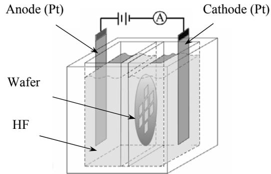
Fig. 3: Schematic of the anodization with HF-ethanol solution.
