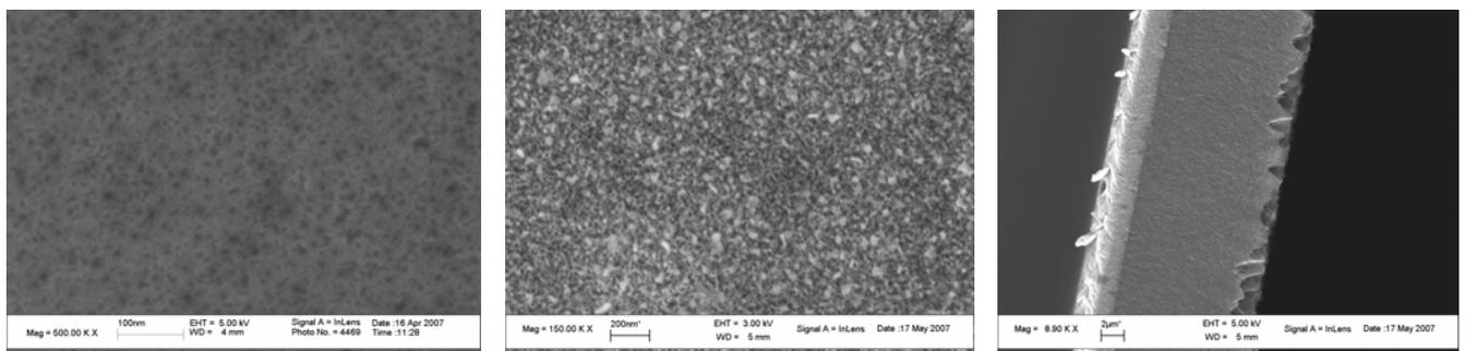
Fig. 6: SEM photos of a permeable porous silicon membrane formed at the current density of 30mA/cm<sup>2</sup>, the HF concentration of 24.5%: (a) the front surface of the membrane, (b) the rear surface of the membrane, and (c) the cross section view of the membrane.
