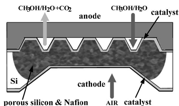
Fig. 1: Schematic of the micro DMFC we proposed, whose flow channels and PEM are formed on one silicon wafer.
