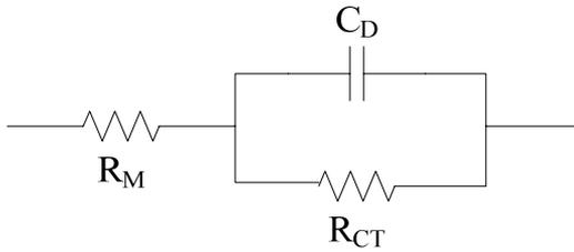
Fig. 7: The equivalent circuit of the porous silicon membrane.
