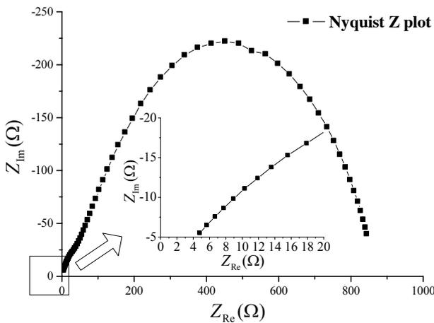
Fig. 8: Nyquist Z plot of impedance of a porous silicon-based membrane, sample 1.
