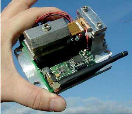
Fig. 2: Integrated piezoelectric vibration energy harvester and wireless temperature and humidity sensing node. (Figure from Ref. [10]).
