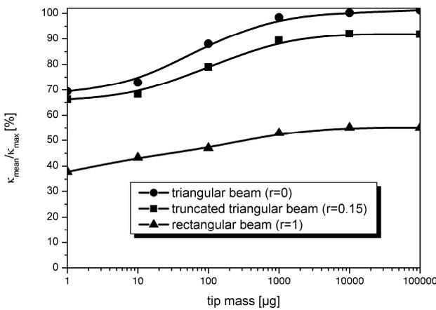
Fig. 6: Theoretical curvature ratio versus tip mass and truncation ratio
