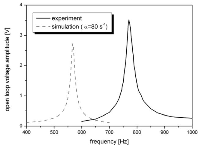
Fig. 8: Measured and simulated first resonance peak of the swivel joint harvester
