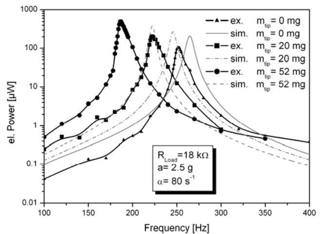
Fig. 5: First resonance of the triangle beam harvester (simulation and experiment)
