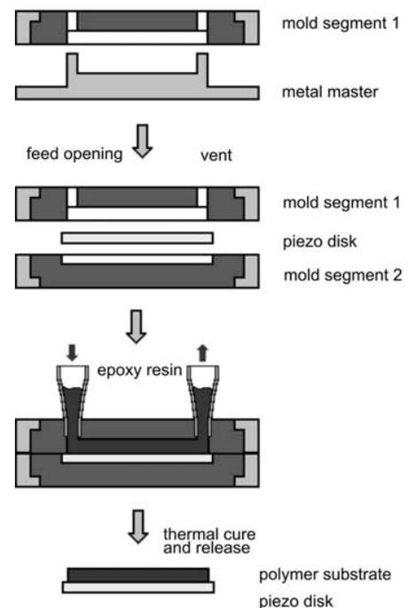
Fig. 1: Process chart of the PPC
