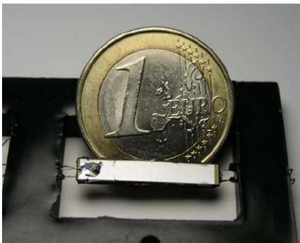
Fig. 7: Photograph of the swivel joint harvester (beam dimensions: 5 mm x 27 mm)
