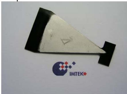
Fig. 3: Photograph of the triangle beam harvester
