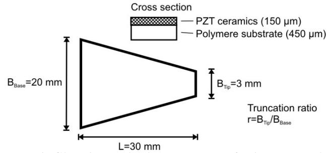
Fig. 4: Sketch and dimensions of the triangle beam harvester
