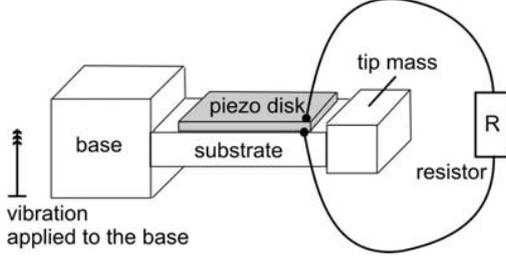
Fig. 2: Generic piezoelectric vibration to electricity converter
