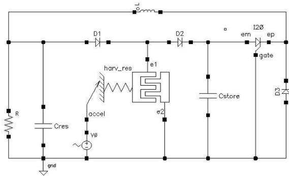
Figure 3: Schematic of the complete harvester model. The devices *harv\_res* and *I20* are modeled in VHDL-AMS.  $L = 2.5 \text{ mH}$ ,  $C_{res} = 1 \mu\text{F}$ ,  $C_{store} = 3.3 \text{ nF}$ .
