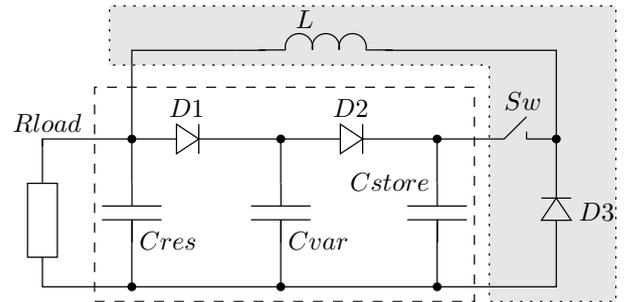
Figure 1: Conditioning circuit of energy harvester inspired from the BUCK DC-DC converter. In dashed frame, the charge pump, in gray, the flyback circuit.
