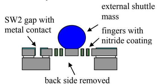
Fig. 8: Cross section view of the fabricated device
