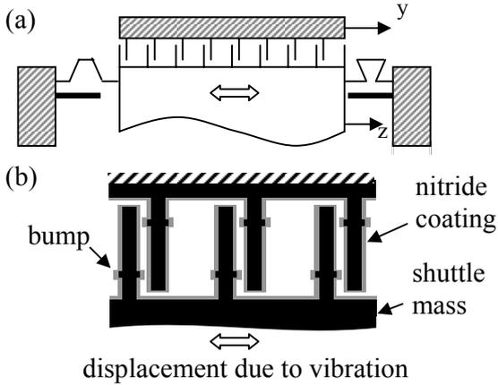
Fig. 2: (a) In-plane gap-closing variable capacitor, (b) bumps on comb fingers
