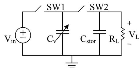
Fig. 1: Operation of the electrostatic energy converter
