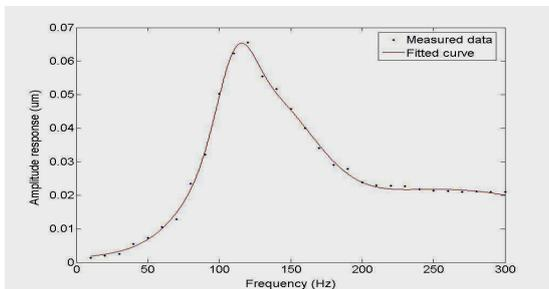
Fig.10: MMA measurement of a device with external mass
