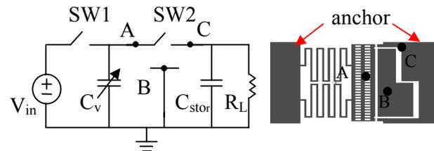
Fig. 5: SW2 as a pull-in contact switch
