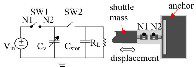
Fig.4 SW1 as a contact mechanical switch
