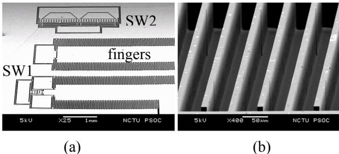
Fig.9: (a) Device overview, showing comb fingers, SW1 and SW2, (b) close-up view of fingers
