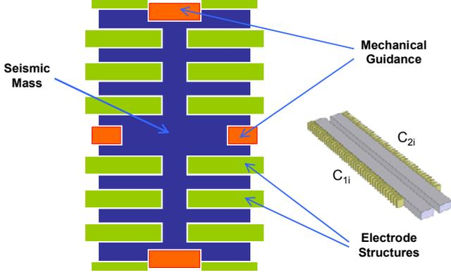
Figure 2: Layout of the micro-generator
