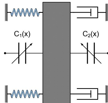
Figure 1: Device concept of the micro-generator
