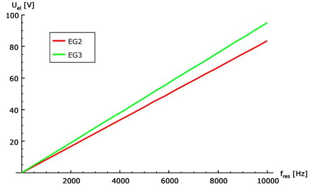
Figure 7: Voltage versus resonance frequency
