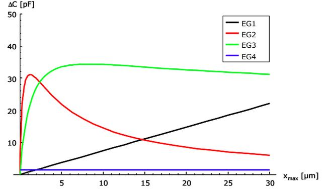
Figure 5: Total change of capacitance versus inner displacement amplitude
