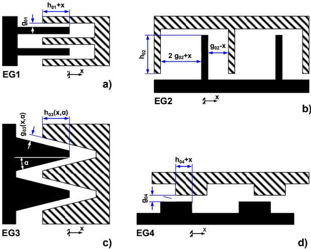
Figure 3: Electrode Designs; a) area-sensitive; b) gap-sensitive; c) angled; d) area-sensitive
