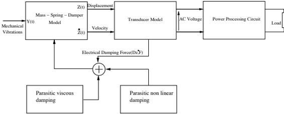
Fig. 2. Block diagram of the generic electromechanical behavior model of the inertial micro generator
