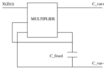
Fig. 4. Generic Variable Capacitor realisation
