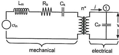
Fig. 1. Equivalent circuit representation of piezoelectric bimorph [1]
