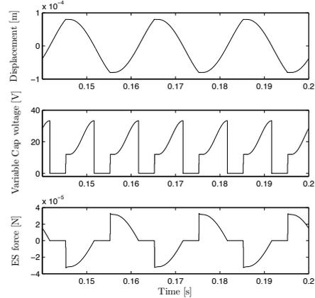
Fig. 7. Inplane gap closing comb drive displacement, variable capacitor voltage and electrostatic force
