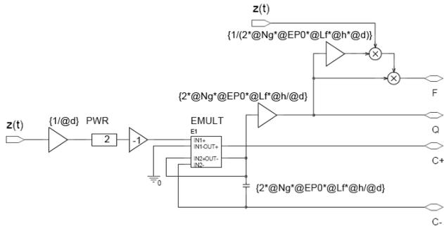
Fig. 5. PSpice model of an inplane gap closing comb drive variable capacitor
