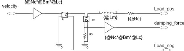
Fig. 3. EM transduction PSpice simulation model
