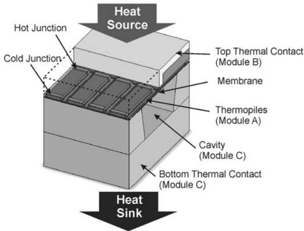
Fig. 1: Schematic of the thermoelectric generator indicating the different fabrication modules.
