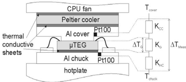
Fig. 6: Schematic of the measurement setup. The thermal network on the right-hand side indicates the contact resistances that consume 85.7% of the measured temperature difference.
