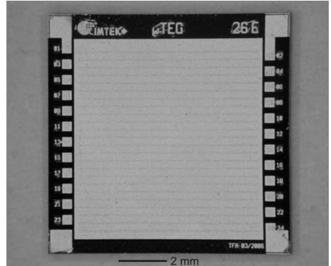
Fig. 5: Microscopic image of the meandering thermocouple structure.
