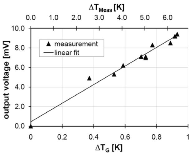
Fig. 7: Measured open-circuit voltage of 125 thermocouples.
