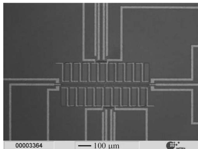
Fig. 3: Microscopic image of the membrane based test structure to measure the Seebeck coefficient.
