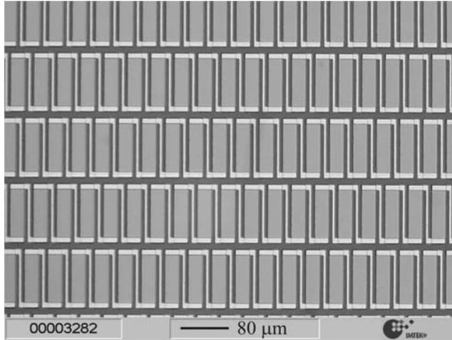
Fig. 4: Microscopic image of the meandering thermocouple structure.
