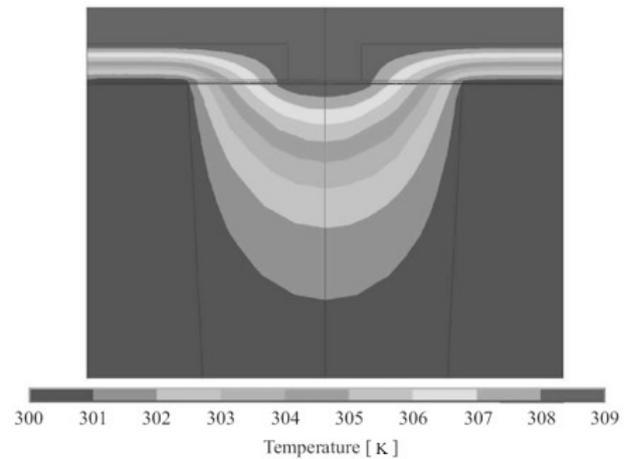
Fig. 2: Temperature distribution within the thermoelectric generator obtained by a 2D FEM thermoelectric simulation with ANSYS.
