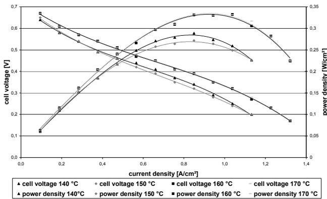
Figure 3: Cell characteristics at different temperatures
