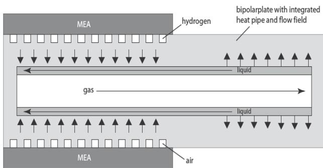
Figure 1: Schematic view of the entity of a fuel cell with integrated heat pipe
