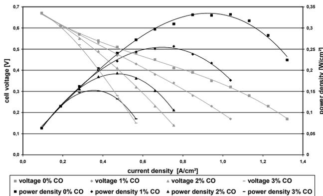
Figure 4: Cell characteristics at different CO fractions in the anode gas (160°C cell temperature)
