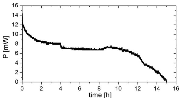
Fig. 7: Power performance of long term measurements of a fully passive DMFC with an anode flow field consisting of 3 parallel double tapered T-shaped channels. Active MEA area (Umicore):  $A_{MEA} = 3 \text{ cm}^2$ .
