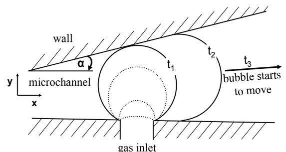
Fig. 2: Schematic time sequence of a growing gas bubble in a tapered channel.
