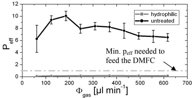
Fig. 6: Pumping performance of double tapered T-shaped channels at various gas flow rates.
