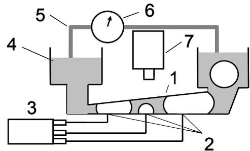
Fig. 5: Experimental set-up for the investigation of pumping efficiencies in double tapered T-shaped structures. (1): Double tapered T-shaped channel (Fig. 3), (2): Six gas inlets evenly distributed at the channel bottom supplied by a syringe pump (3) (Braun Melsungen), (4): Reservoir, (5): Tube, (6): Flow sensor (Sensirion) (7): Camera (Phillips webcam).
