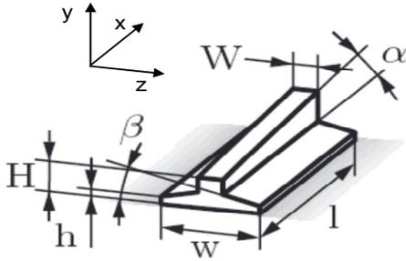
Fig. 3: Investigated double tapered T-shaped channel structure.  $W = 800 \mu\text{m}$ ,  $w = 3000 \mu\text{m}$ ,  $H = 800 \mu\text{m}$ ,  $h = 300 \mu\text{m}$ ,  $l = 20000 \mu\text{m}$ ,  $\alpha = 3^\circ$ ,  $\beta = 7^\circ$ .
