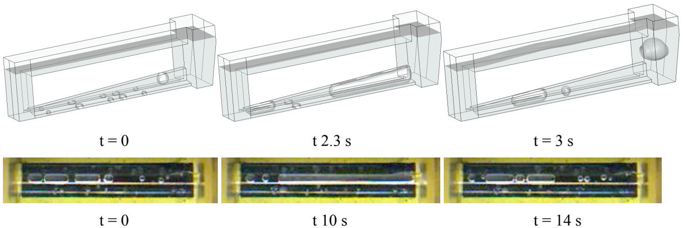
Fig. 4: Time sequence of growing and moving bubbles in double tapered T-shaped channels ( $\alpha = 3^\circ$ ,  $\beta = 7^\circ$ ) during DMFC operation. Top: CFD simulation ( $\Phi_{\text{gas}} = 320 \mu\text{L min}^{-1}$ ) Bottom: Fuel cell experiments.  $\Phi_{\text{gas}} \approx 51 \mu\text{L min}^{-1}$ .
