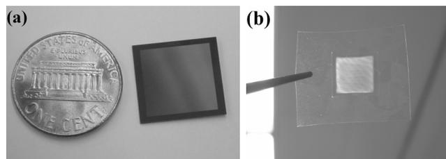
Fig. 1 View of (a) the prepared mould for the nanoimprint procedure and (b) the nanoimprinted Nafion<sup>®</sup> 117 membrane.
