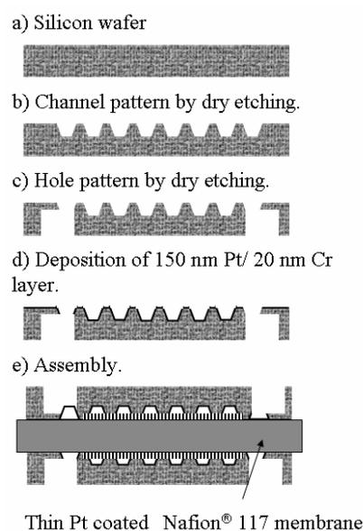
Fig. 2 Fabrication sequence of MEMS-based micro DMFC.
