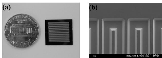
Fig. 3 (a) View of the prepared Pt-coated Si separator. (b) SEM image of the prepared trapezoid channel structure.
