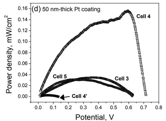
Fig. 5 Measured performances of the prepared MEMS-based DMFCs. Cell 1' and Cell 4' were of the same nanoimprinted pattern as Cell 1 and 4 except that the nanoimprint procedure was after the deposition of Pt film.
