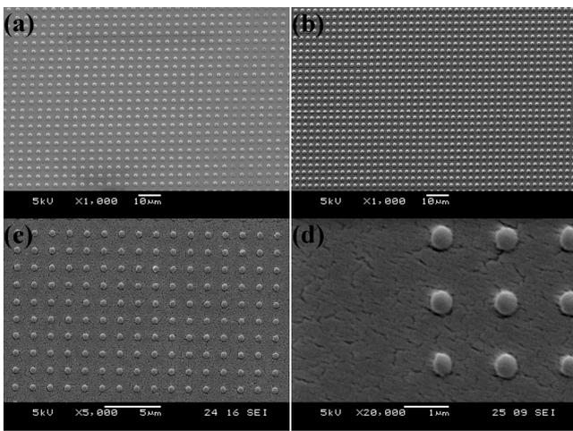
Fig. 4 SEM images of the nanoimprinted patterns consisting of micro convex with (a) 2  $\mu\text{m}$ -in-diameter and 2  $\mu\text{m}$ -in-spacing, (b) 2  $\mu\text{m}$ -in-diameter and 1  $\mu\text{m}$ -in-spacing, (c) and (d) 0.5  $\mu\text{m}$ -in-diameter and 1  $\mu\text{m}$ -in-spacing.
