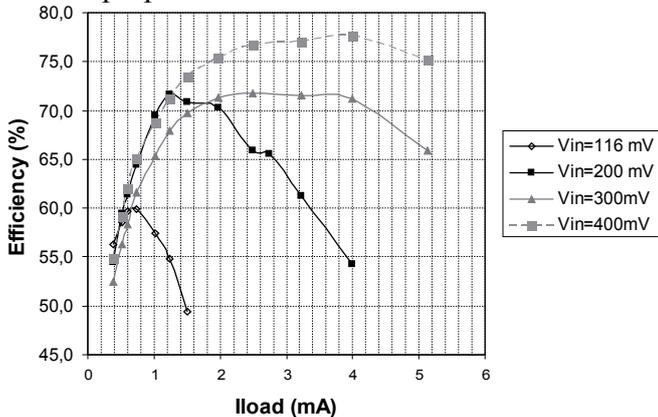
Fig. 6. Measured efficiency vs. load current for different input voltages.
