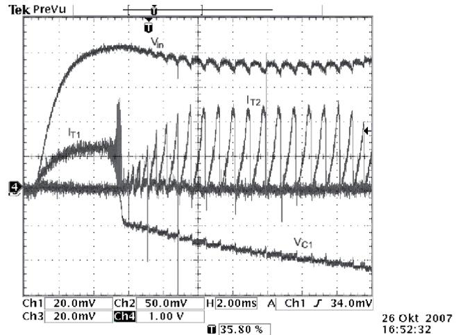
Fig. 4. Measured waveforms obtained during the start-up phase. Ch1 corresponds to  $I_{T2}$ , Ch2 to  $V_{in}$ , Ch3 to  $I_{T1}$  and Ch4 to  $V_{C1}$ .
