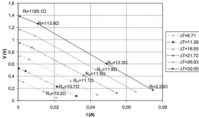
Fig. 1. Measured output voltage of the TEG as a function of current for different  $\Delta T$  values.  $R_m$  is the internal resistance of the TEG and  $R_l$  is the value of the different resistive loads connected to the TEG.
