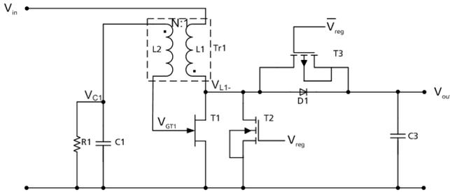
Fig. 3. Simplified schematic of the power management unit based on coupled inductors.
