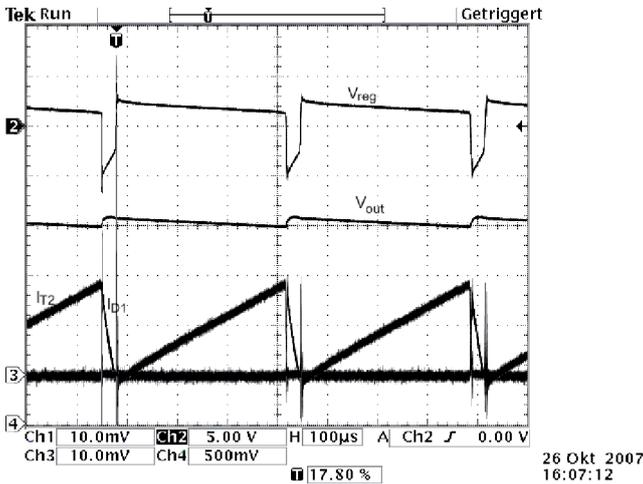
Fig. 5. Measured waveforms obtained during the steady-state phase. Ch1 corresponds to  $I_{T2}$ , Ch2 to  $V_{GR2}$ , Ch3 to  $I_{D1}$  and Ch4 to  $V_{out}$ .
