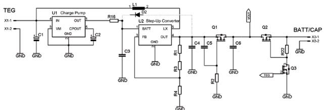
Fig. 2. Schematic of the power management unit composed by a charge-pump and a step-up converter.
