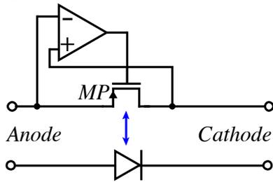
Fig. 5: Circuit diagram of the proposed active diode (AD) with comparator and switch *MP*.
