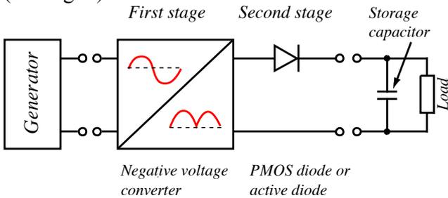
Fig. 3: Proposed two stage rectifier with first stage (negative voltage converter) and second stage (diode part).
