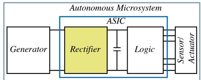
Fig. 1: Schematic of an autonomous microsystem with CMOS integrated rectifier.
