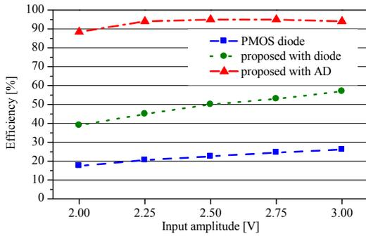
Fig. 7: Efficiency of different rectifiers versus the input amplitude.
