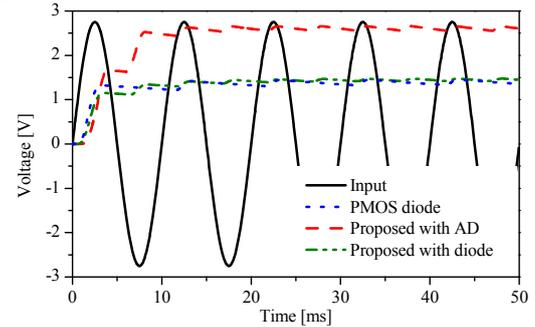
Fig. 6: Input and output wave forms of different rectifiers.
