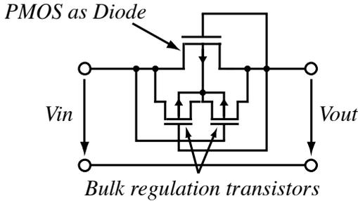
Fig. 2: Circuit diagram of a PMOS transistor connected as diode and the bulk regulation transistors.
