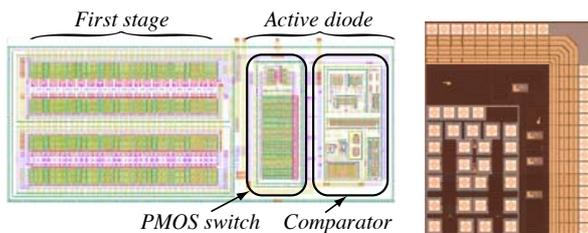
Fig. 8: Layout of the proposed rectifier ( $250 \times 100\ \mu\text{m}^2$ ) and micrograph of the CMOS chip.
