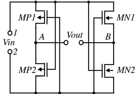
Fig. 4: Circuit diagram of the first stage (negative voltage converter).
