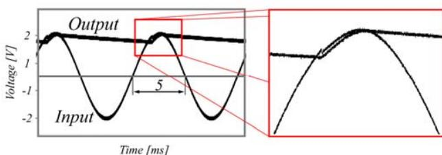
Fig. 9: Measured input and output wave form of the active diode.
