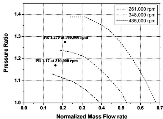
Fig. 10: Compressor test results vs. Design values
