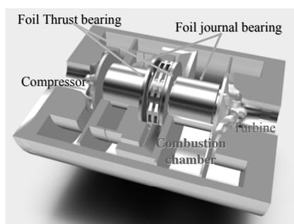
Fig. 1: 100watts class micro gas turbine engine
