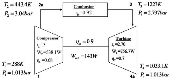
Fig. 2: Micro gas turbine cycle analysis
