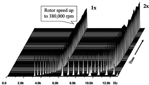
Fig. 8: Waterfall frequency spectrum at startup
