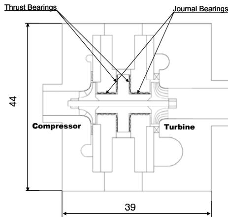
Fig. 3: Cross section of the micro turbocharger
