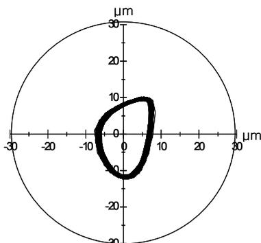
Fig. 9: Orbit at the rotational speed 380,000 rpm
