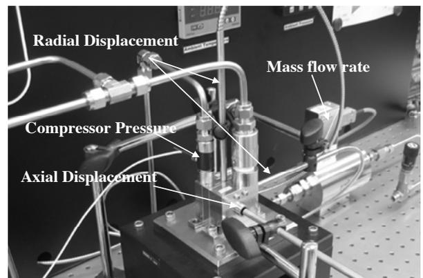
Fig. 7: Test rig setup
