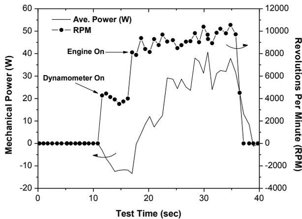
Figure 3: Positive power is generated for a naturally aspirated operation of the S1500 engine. The engine produces a peak power of 40.6 W at 9600 rpm.
