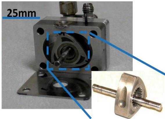
Figure 1: Liquid fuel operated side ported S1500 rotary engine, and rotor with an inverted teardrop-shaped combustion pocket.
