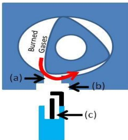
Figure 5: The path of blow-by is open when the rotor passes the spark plug hole: (a) Spark plug recess, (b) Spark plug hole, (c) Dead volume in spark plug.
