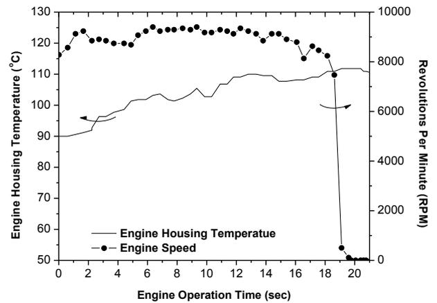
Figure 4: Measurement of the housing temperature of the S1500 engine, which provides a measure to determine the combustion efficiency.
