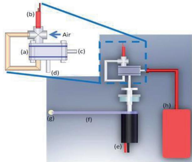
Figure 2: Schematic of the engine performance test setup: (a) S1500 engine, (b) Liquid fuel injector, (c) Ignitor, (d) Shaft, (e) Universal dynamometer, (f) Torque arm, (g) Load cell, (h) Ignition system.
