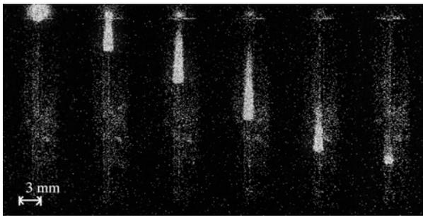
Fig. 5:  $\text{OH}^*$  chemiluminescence of oscillating flame in the 0.7-mm-thick combustion channel. Optical band-pass filter at 307 nm is employed.
