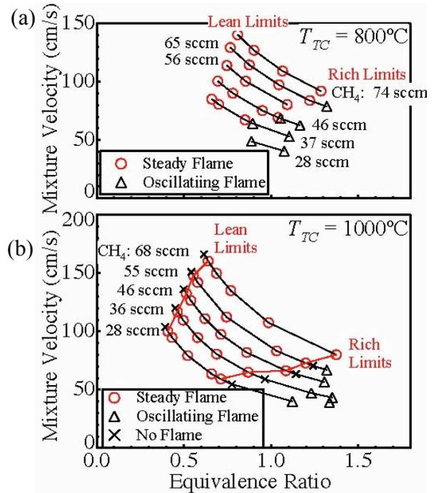
Fig. 7: Flammability limits in the 0.7-mm-thick combustion channel. (a)  $T_{TC} = 800^{\circ}\text{C}$ , (b)  $T_{TC} = 1000^{\circ}\text{C}$ .
