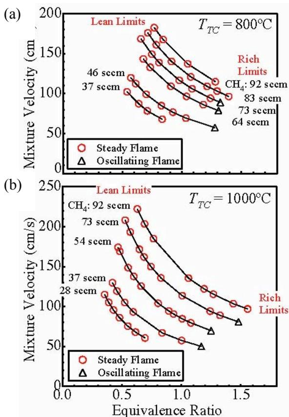
Fig. 8: Flammability limits in the 1.0-mm-thick channel. (a)  $T_{TC} = 800^{\circ}\text{C}$ , (b)  $T_{TC} = 1000^{\circ}\text{C}$ .
