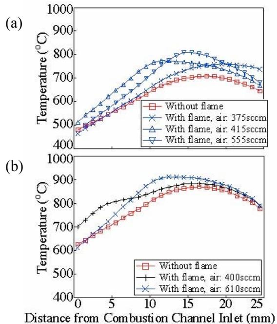
Fig. 3: Temperature profile along the centerline of the combustion channel at the sidewall outer surface. CH<sub>4</sub> flow rate is 45.6 sccm. (a)  $T_{TC}=800^\circ\text{C}$ ; (b)  $T_{TC}=1000^\circ\text{C}$ .
