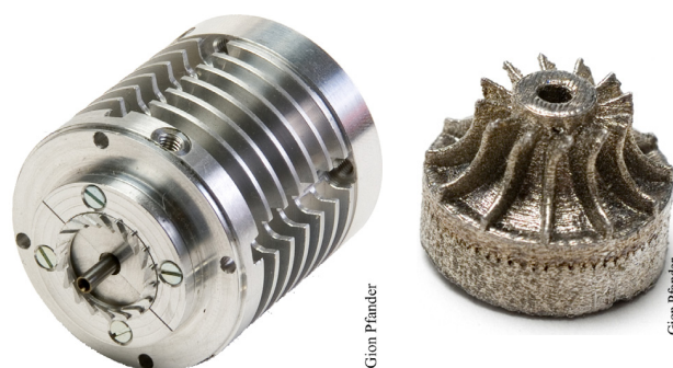
Fig. 2. PM Generator with stator guide vanes and the radial-flow turbine ( d = 10.5 mm).
