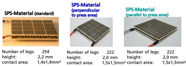
Fig. 10: Thermoelectric modules with preferential orientation (not oriented modules of the first generation (left) are compared to more recent modules, where the n-type legs are oriented in parallel (right) or perpendicular (middle) to the wafer surface).
