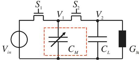
Figure 2: Electrical harvesting circuit for a variable capacitor (diodes may be used as passive switches).
