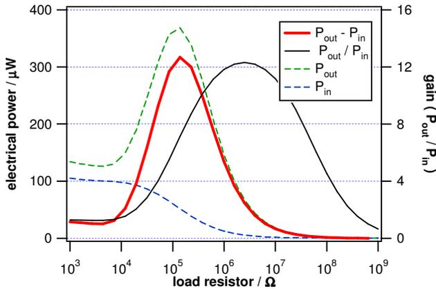
Figure 10: Matching the energy scavenger with a resistive load. In the present case maximum power is obtained for a load of 140 kΩ. Optimum utilization of the provided electrical power occurs at 2.5 MΩ.
