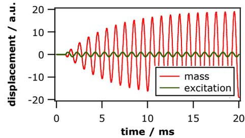
Figure 4: Motion of the suspended seismic mass under the influence of viscous damping.
