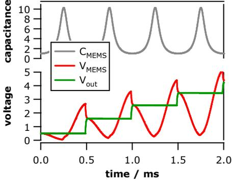
Figure 6: Capacitance change and voltage of the circuit shown in Figure 2. The incremental charge transfer increases the output voltage gradually.
