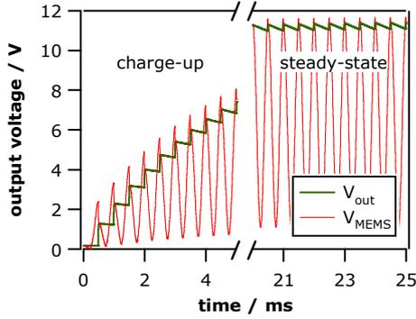
Figure 7: Saturation of output with an input voltage of 1 V.
