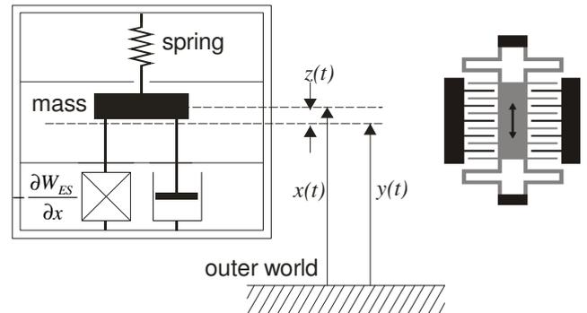
Figure 1: (left) Lumped mechanical model of the resonant scavenger including non-linear electrostatic and viscous damping. (right) schematic representation of a gap-closing electrostatic scavenger.
