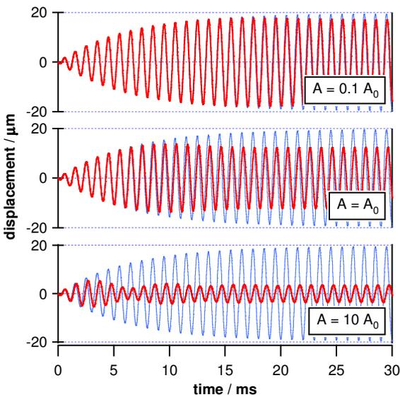
Figure 11: Effect of electrostatic damping on the amplitude. In contrast to purely mechanically damped motion (blue) the biasing voltage ( $V_{in} = 1$  V) may strongly damp the motion of the mass (red) depending on the capacitor area  $A$ .
