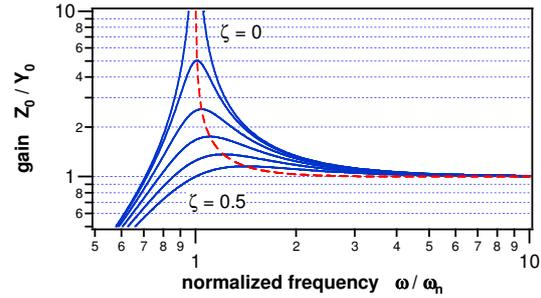
Figure 3: Gain curves for a resonator with linear damping (normalized damping coefficient  $\zeta = d/2m\omega_n$ ).
