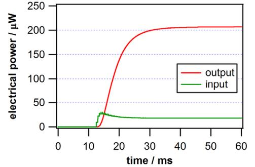
Figure 9: Initial phase of the energy scavenging process. Initially electrical power has to be drawn from the voltage source for repeatedly charging the variable capacitor.
