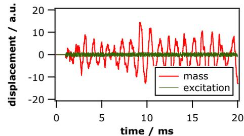
Figure 5: Resultant motion of the mass under broadband excitation (bandwidth limited white noise spectrum).
