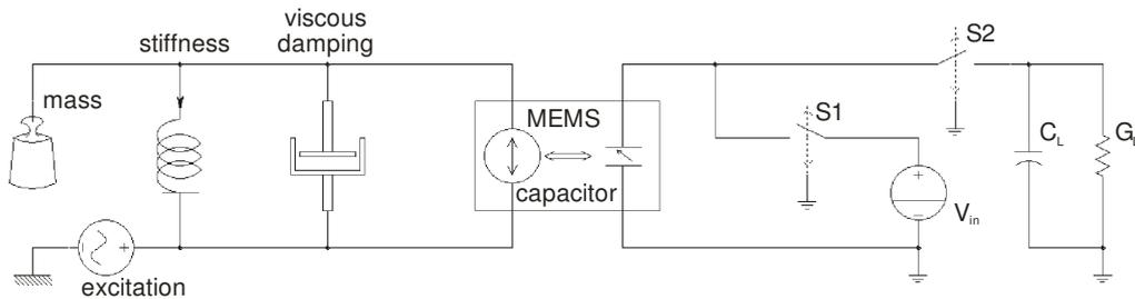
Figure 8: Simplified behavioral model for the energy scavenger. An electro-mechanical model of the variable capacitor couples the mechanical domain (left) with the harvesting circuitry (right). The logic for controlling the switches is not shown.
