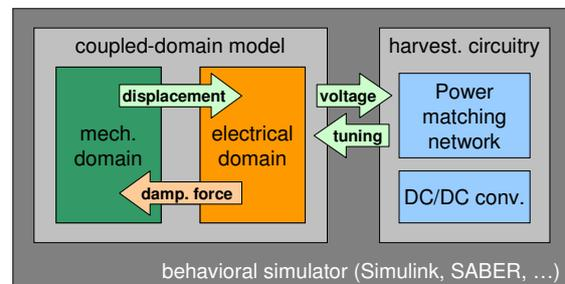
Figure 12: Interaction of the coupled-domain scavenger model and accompanying harvesting circuitry within a single design environment
