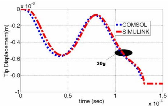
Figure 2: Cantilever tip deflection under 0.95 V and 30g shock loading (zero damping).
