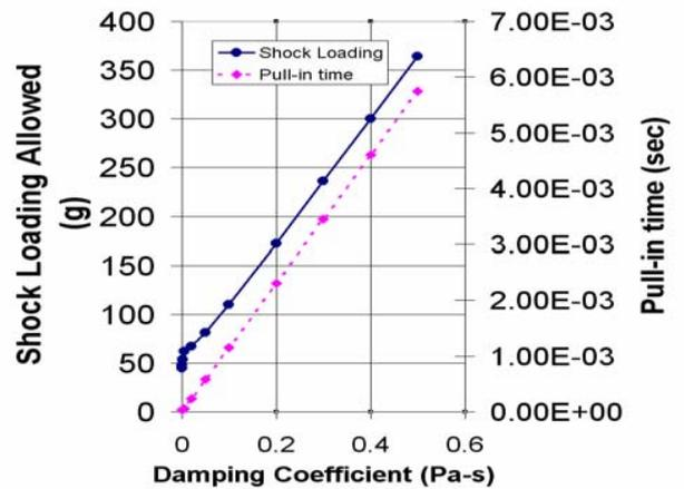
Figure 4: Threshold shock loading and pull-in time as a function damping coefficient
