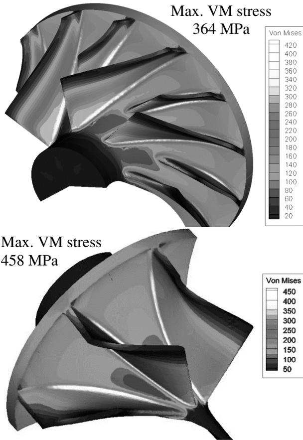
Fig. 4. Von Mises stresses in the optimised compressor (top) and turbine (bottom) geometries.
