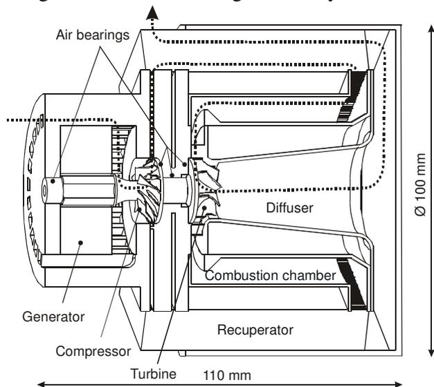
Fig. 1: Gas turbine generator layout.
