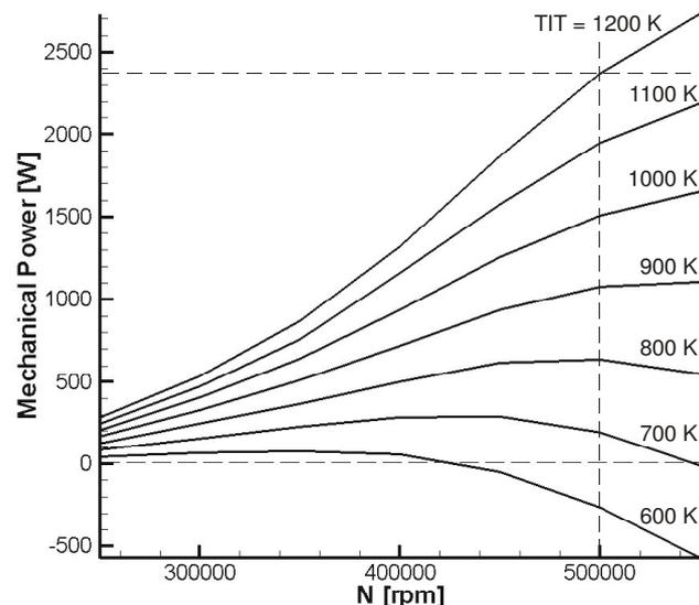
Fig. 2: Mechanical power vs. speed and turbine inlet temperature (TIT) (without recuperator).
