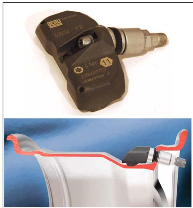
Fig. 1: A TPMS module. Top – image of a module. Bottom – indication of how a module sits on the rim. Courtesy of Beru AG.
