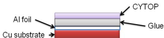
Fig. 5: The structure that enables a film of CYTOP electret material to be peeled-off from a substrate. The aluminum foil is inserted so that the hard copper substrate can be removed before the peeling-off process. Both glue and CYTOP are liquids before heat-solidification treatments, and they are spin-coated during the process.
