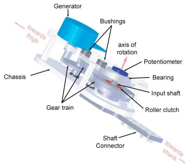
Fig. 2: A schematic of the chassis illustrates the location of transmission, generator and sensing components.
