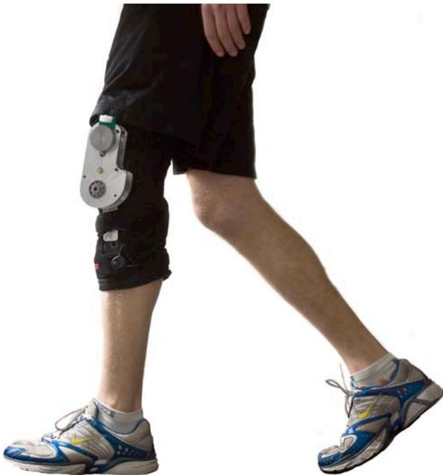
*Fig. 3: The device consists of an aluminum chassis and generator mounted on an orthopedic knee brace. The entire unit weighs 1.6 kg. While the subject in this image is wearing the device only on his left leg, all subjects were tested with devices worn bilaterally.*
