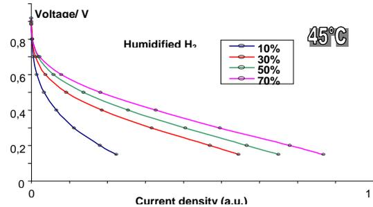
Figure 6. Polarization curves of a microfuel cell running with passive air-breathing system in different relative humidities. Humidified Hydrogen,  $T^{\circ}=45^{\circ}\text{C}$ .
