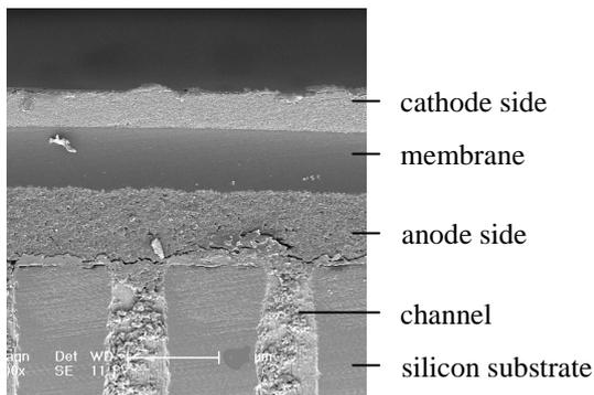
Figure 2. SEM picture of a micro fuel cell.
