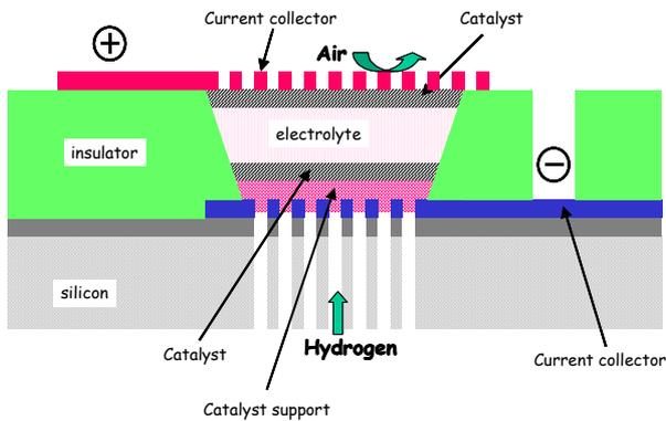
Figure 1. Schematical view of the CEA/ST microPEMFC.
