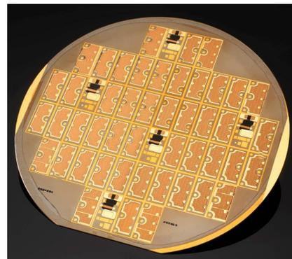
Figure 3. Fuel cells on a 200 mm wafer : each golden dot is a single fuel cell core
