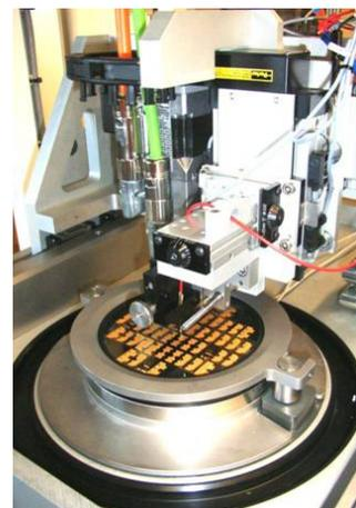
Figure 4. Micro fuel cell test system.
