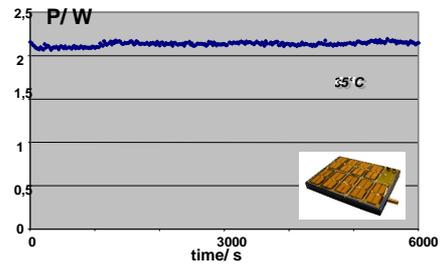
Figure 8. Evolution of the power density versus operating time of a prototype (potentiostatic mode).
