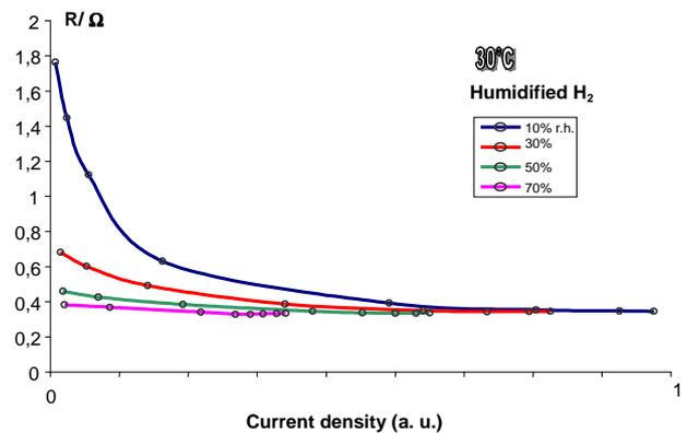
Figure 7. Internal resistance versus current density for a micro fuel cell running with passive air-breathing system in different relative humidities. Humidified Hydrogen,  $T^{\circ}=30^{\circ}\text{C}$ .
