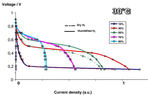
Figure 5. Polarization curves of a microfuel cell running with passive air-breathing system in different relative humidities. Dry Hydrogen: dotted line, humidified Hydrogen : solid line,  $T^{\circ}=30^{\circ}\text{C}$ .
