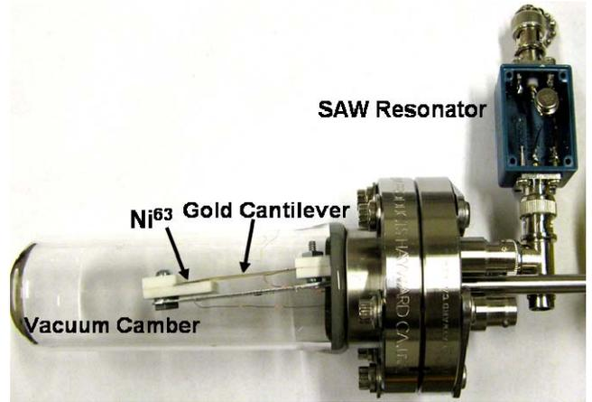
Figure 6. Photograph of the prototype radioisotope-powered SAW transponder
