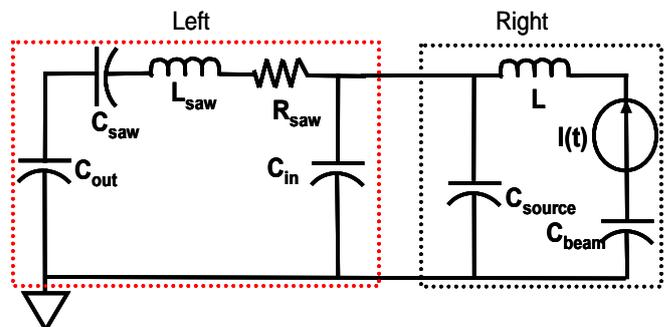
Figure 4. The equivalent circuit model of the SAW transponder
