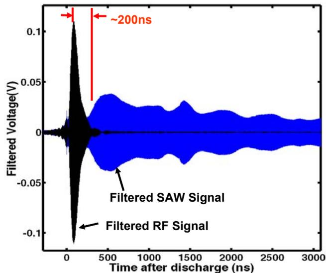
Figure.9 Bandpass-filtered signals illustrating the SAW resonator signal delay
