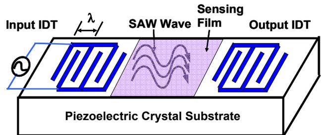
Figure 3. Schematic illustrating operation principle of the SAW resonator
