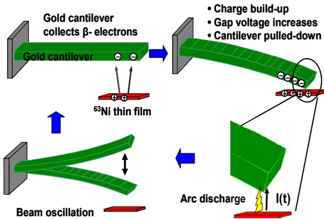
Figure 2. Schematic illustrating the radioisotope actuated reciprocation of gold cantilevers.
