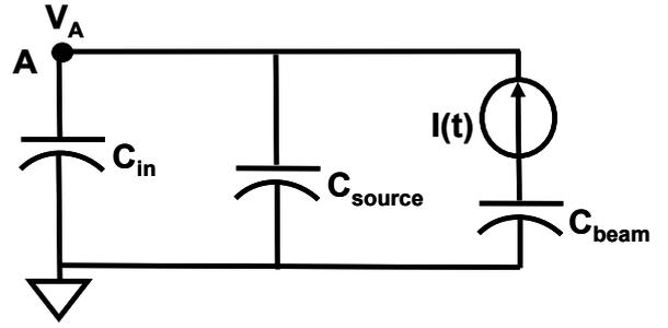
Figure 5. Simplified equivalent circuit model of the SAW transponder during charging process
