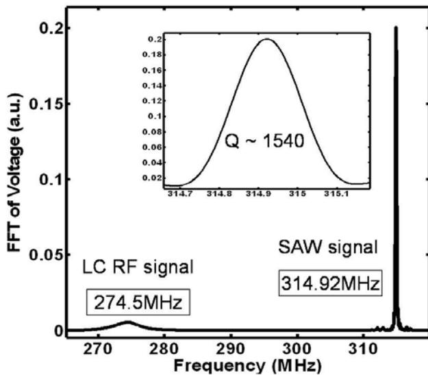
Figure. 8 Frequency of the RF signal with 315MHz Saw resonator connected
