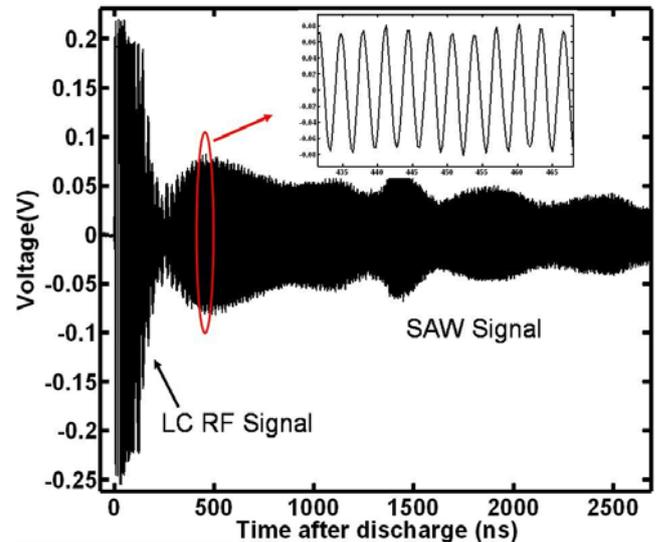
Figure. 7 Measured RF signal waveform with 315MHz SAW resonator connected
