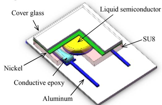
*Fig. 1: 3D view of the micromachined liquid semiconductor diode as a thermal harvester.*
