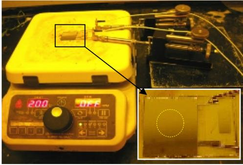
Fig. 4: Picture of the fabricated thermal harvester and the experimental set up.
