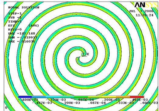
Fig. 5: Open circuit electric field in the middle plane of PZT film with 5g acceleration in x-direction.
