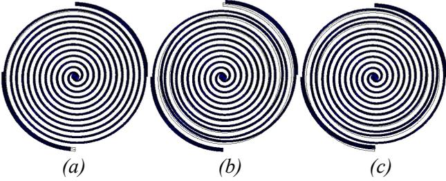
Fig. 2: The 1-3 modes of the SPEH vibration in-plane.
