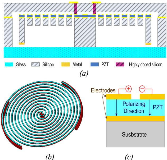
Fig. 1: Schematic structure of the SPEH working in-plane: (a) side view; (b) perspective drawing; electrode configuration.
