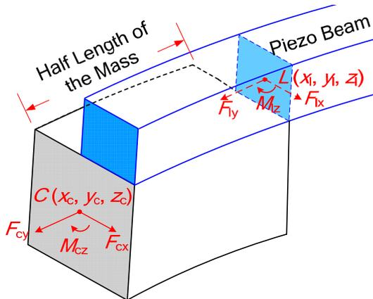
Fig. 3: Schematic of the spiral beam connected with the large proof mass.
