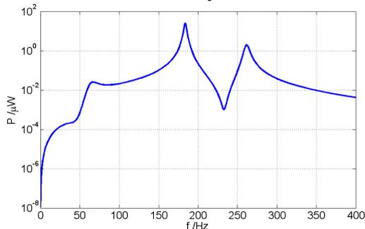
Fig. 6: The output power of the SPEH under acceleration with the amplitude of 5g, and load resistance 630k $\Omega$ .
