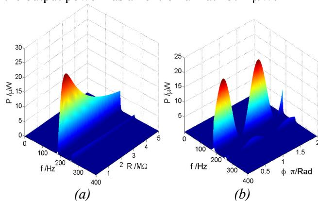
Fig. 7: The output power of the SPEH versus (a) resistance load with  $\phi=\pi/2$ ; (b) the direction of external acceleration with  $R=630k\Omega$ .
