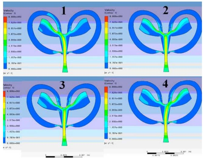
Figure 2: Simulation of Coanda fluidic oscillator design: Velocity profile coded by shading in the inside of geometry. The jet from below attaches to the left and right walls alternatively.
