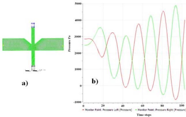
Figure 8: a) Meshed simulation model of the edgetone generator. b) Pressure in the edgetone generator chambers over time when there is a pressure difference of  $\Delta p = 5kPa$  between input and output. The simulation shows an oscillation frequency of around 4kHz.
