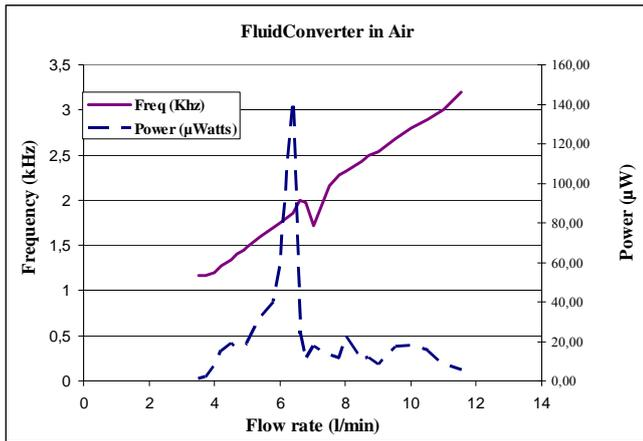
Figure 4: Oscillation frequency and electrical power output over flow rate in the prototyped oscillator mode in air. The preliminary measurement data shows a small notch in the frequency response that may be attributed to a measurement error.
