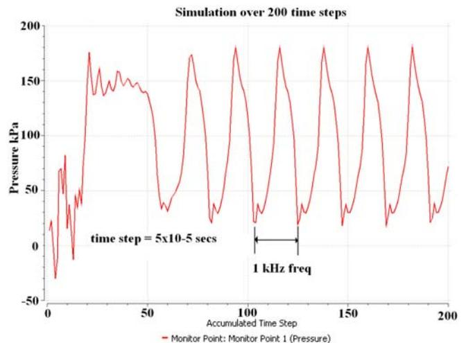
Figure 3: Simulation: Air pressure over time in one of the oscillator feedback arms at a flow rate of 5 l/min. See the agreement with model results in Figure 4.
