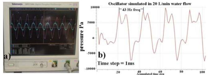
Figure 6 : a) Voltage output of the two piezoelectric chambers over time. The flow rate is 20l/min water. Frequency is 45Hz (time interval shown on screen is 200ms). b) Pressure over time in feedback channel of the Coanda fluidic oscillator when simulated in water at a flow rate of 20l/min. Pressure oscillates at 43Hz.
