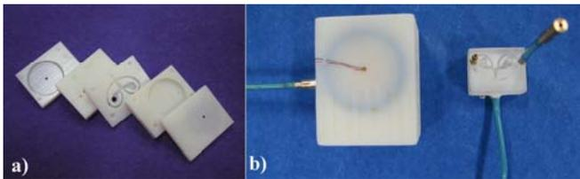
Figure 5: a) Exploded view of a fluidic oscillator design with integrated piezoelectric chambers (circular disks over and under the oscillator). b) Integrated design on the left in comparison to the first working prototype for air on the right.
