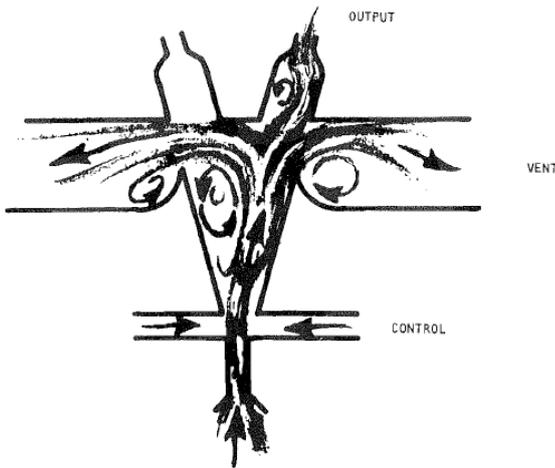
Figure 1: Coanda effect in a bistable switch: A jet enters the nozzle below and is deflected to either wall and exists in one of the two outputs or vents. A control signal from the side can deflect the jet (from [1]).
