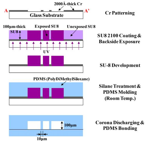
Fig. 4: Fabrication process of the pressure compensation valves at the cross-section A-A' in Fig.3.
