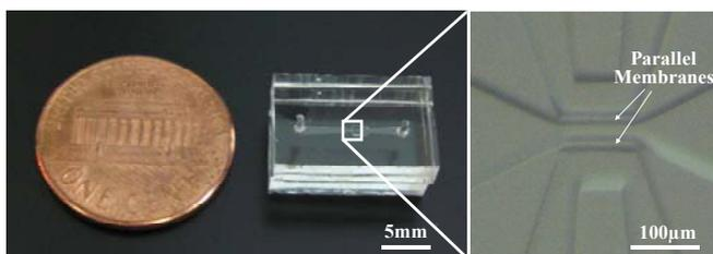
Fig. 5: Fabricated prototype with an enlarged view of the parallel membranes.
