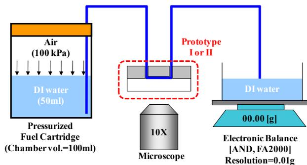
Fig. 6: Experimental setup for flow-rate measurement using DI water as a fuel.
