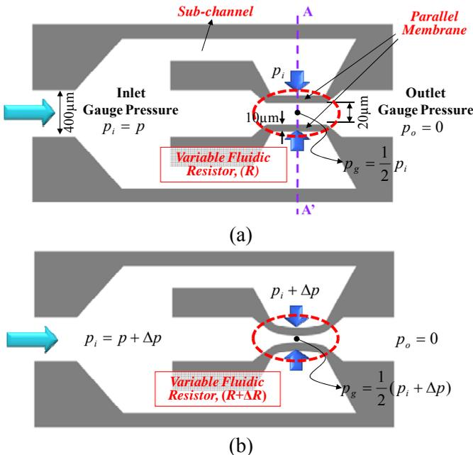
Fig. 3: Working principle of flow-rate regulators [5] using the autonomous deflection of parallel membrane valves: (a) for the inlet pressure,  $p_i$ ; (b) for the increased inlet pressure,  $p_i+\Delta p$ .
