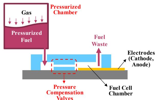
Fig. 1: Schematic view of the present pumpless fuel supply method using pressurized fuel regulated by passive pressure compensation valves.
