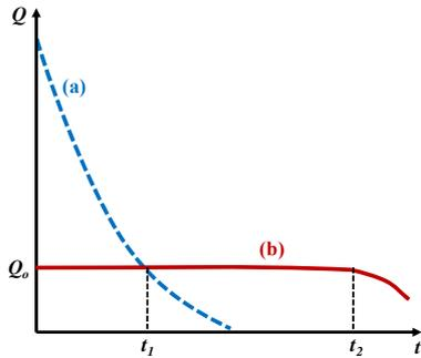
Fig. 2: Comparison of fuel flow-rate ( $Q$ ): (a) flow-rate using pressurized fuel only; (b) flow-rate using the pressurized fuel regulated by the passive pressure compensation valves.
