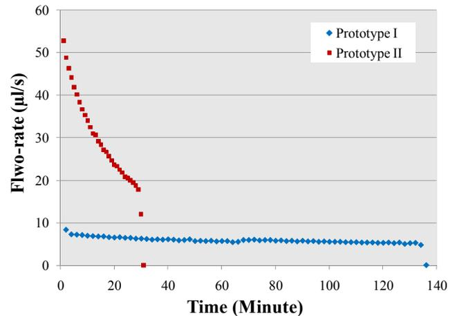
Fig. 7: Measured DI water flow-rate of the prototype I (with pressure compensation valves) and II (without pressure compensation valves). Both prototypes are connected to the identical pressurized chamber (100ml), filled with DI water (50ml) and pressurized upto 100 kPa by air.
