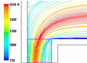
Fig. 4: Outlet peak temperature and recirculation zone: Pathlines colored by static temperature (K)
