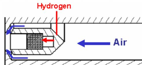
Fig. 2: "Inverse Micromix" injector: working principle
