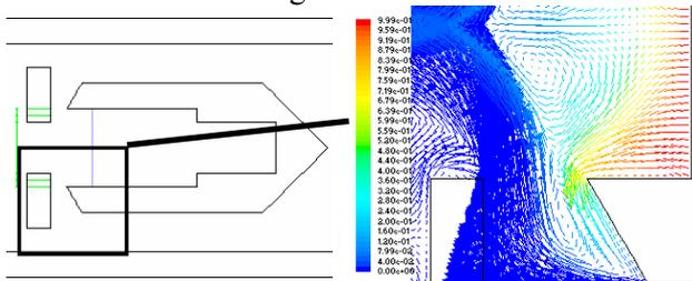
Fig. 3: Injection system with deviation plates
