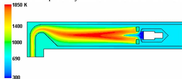
Fig. 5: Static temperature on the optimized geometry
