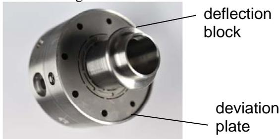
Fig. 7: Annular test chamber without outer wall
