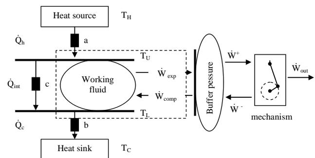
Fig. 1: Generic Stirling machine scheme
