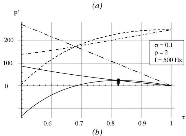
Fig.4 Power balance with respect to temperature ratio
