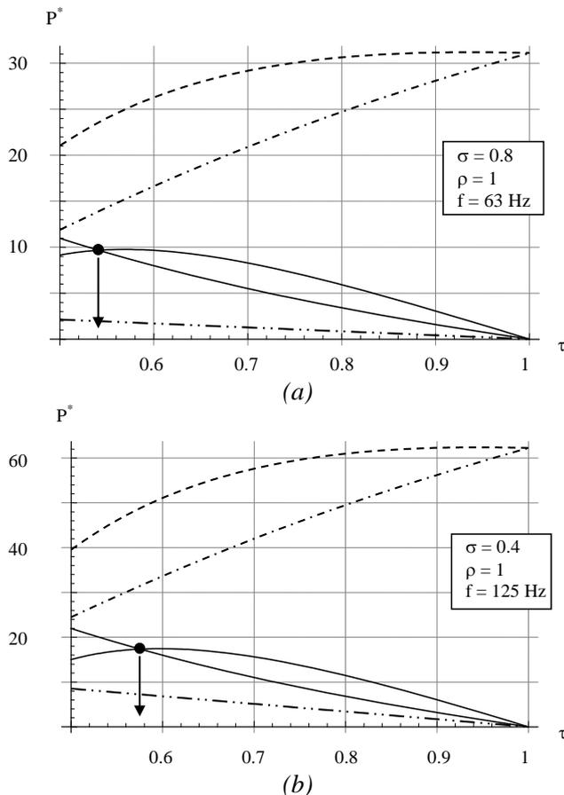
Fig.3 Power balance with respect to temperature ratio
