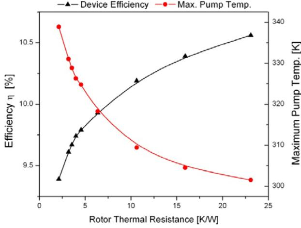
Fig. 4: Effect of the rotor thermal resistance on the thermal efficiency and the maximum pump temperature.
