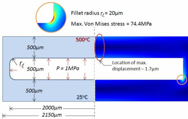
**Fig. 6:** Schematic and results of a coupled thermal & mechanical finite element model of a fused silica static structure.
