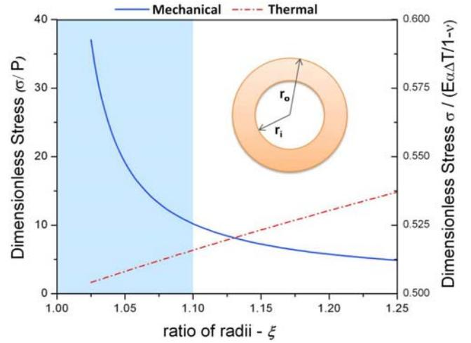
Fig. 5: Variation of thermal and mechanical stress as a function of the ratio of radii.
