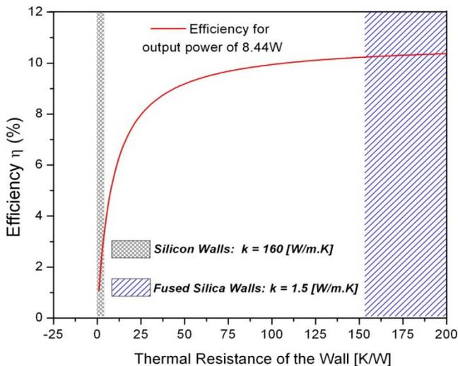
**Fig. 2:** Effect of the thermal resistance of the static walls on the thermal efficiency of a Rankine microturbine, showing that low conductivity materials (such as fused silica) are required for acceptable device efficiency.
