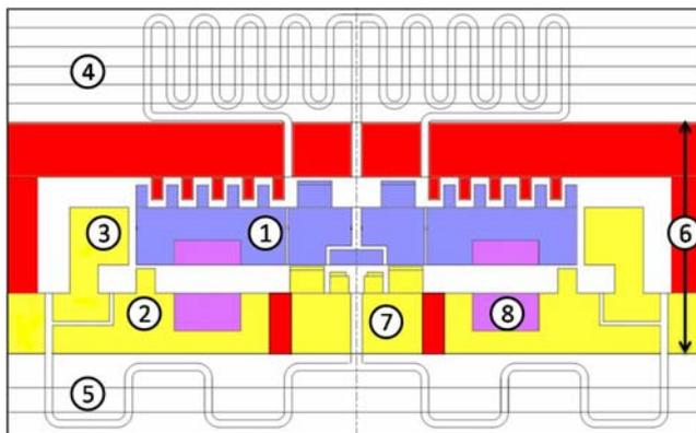
**Fig. 1:** Schematic cross-section of a Rankine microturbine: (1) rotor, (2) thrust bearing, (3) journal bearing, (4) evaporator, (5) condenser, (6) static structure, (7) pump, and (8) generator. The structure is ~1 mm in thickness and ~10 mm in diameter.
