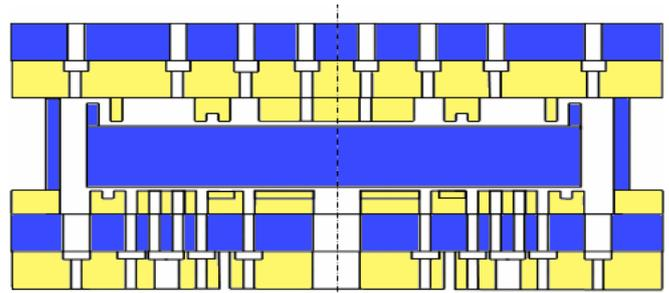
**Fig. 7:** Schematic representation of the turbine holding the pump, fused silica is in blue, silicon is in yellow
