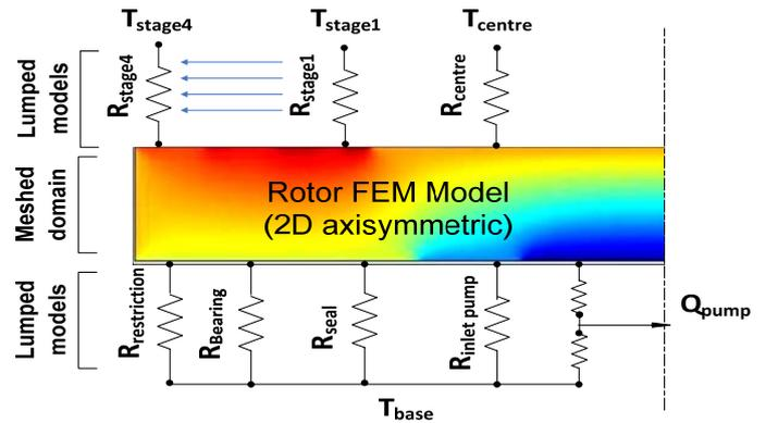
**Fig. 3:** Scheme of coupled heat transfer model approach consisting of discretized FEM for the rotor surrounded by lumped models for the components.
