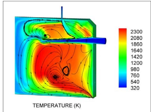
Figure 4: 3D fields for temperature and stream lines.
