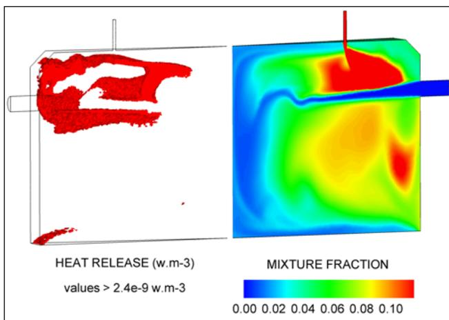
Figure 3: 3D fields for heat release and mixture fraction.
