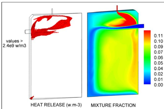
Figure 5: 3D fields for heat release and mixture fraction.
