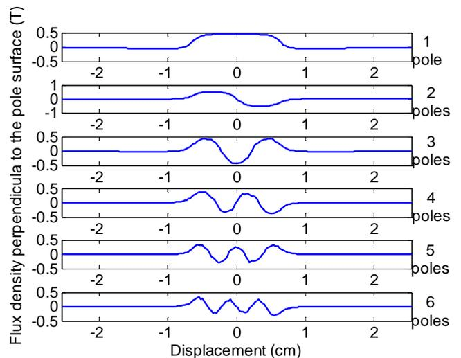
Fig. 2: Flux density profiles of array configurations with 1-6 magnets (1mm air gap).
