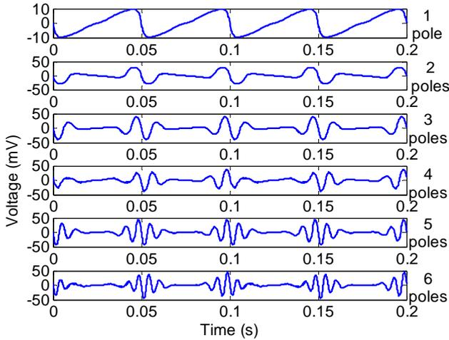
Fig. 3: Open circuit voltage waveforms of array configurations with 1-6 poles (air gap of 1mm).
