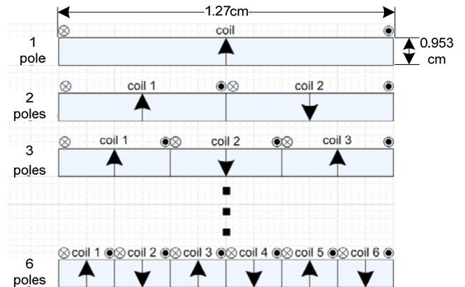
Fig. 1: Schematic cross-section of magnetic array simulation (extends 2.54 cm out of the plane).
