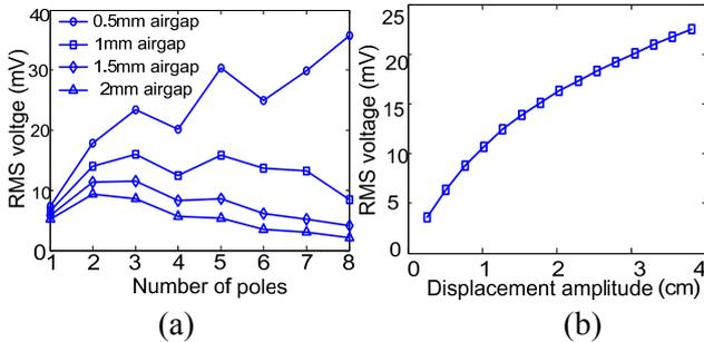
Fig. 4: (a) RMS voltage vs. number of poles with different air gaps. (b) RMS voltage vs. displacement amplitude (4 poles; 1 mm air gap).
