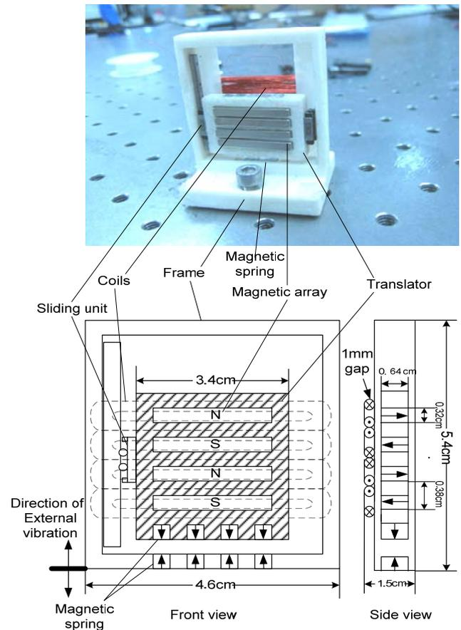
Fig. 5: Picture and schematic of the prototype.
