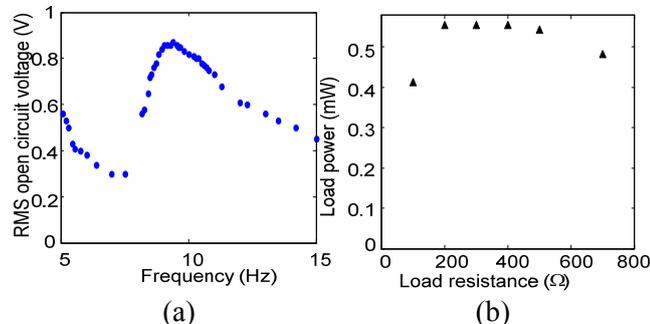
Fig. 7: (a) RMS open-circuit voltage vs. excitation frequency at 0.8 g and (b) Load power vs. load resistance at 0.8 g and 9.2 Hz.
