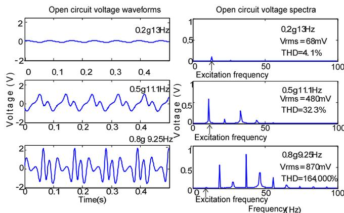
Fig. 6: Open-circuit voltage waveforms and frequency spectra showing voltage enhancement and frequency multiplication with increasing excitation level. Rms voltage and total harmonic distortion (referenced to the input waveform frequency) are summarized within the plots.
