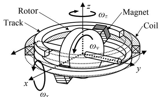
Fig.1 : Structure of gyroscopic generator.
