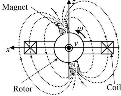
Fig 3 : Magnetic-field distribution.
