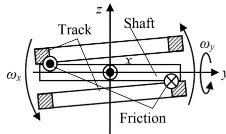
Fig. 2 : Principle for increase of spinning velocity.
