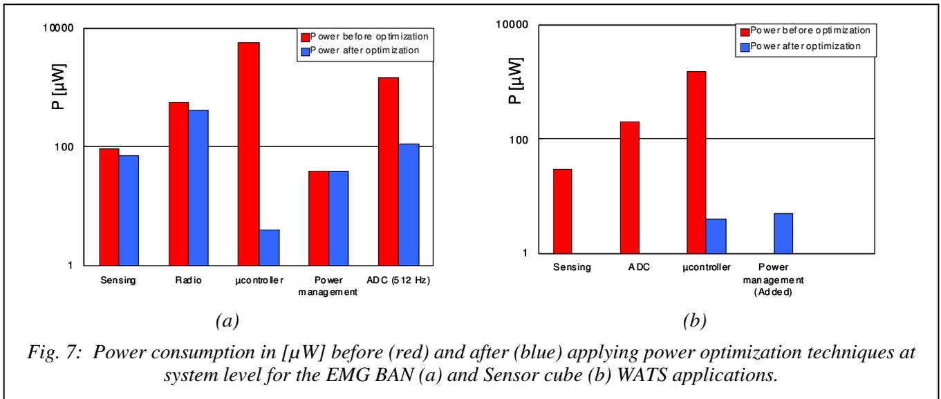
Fig. 7: Power consumption in  $[\mu\text{W}]$  before (red) and after (blue) applying power optimization techniques at system level for the EMG BAN (a) and Sensor cube (b) WATS applications.
