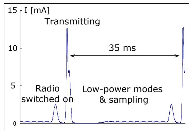
*Fig. 6: Current consumption and duty-cycle for the BAN EMG application.*
