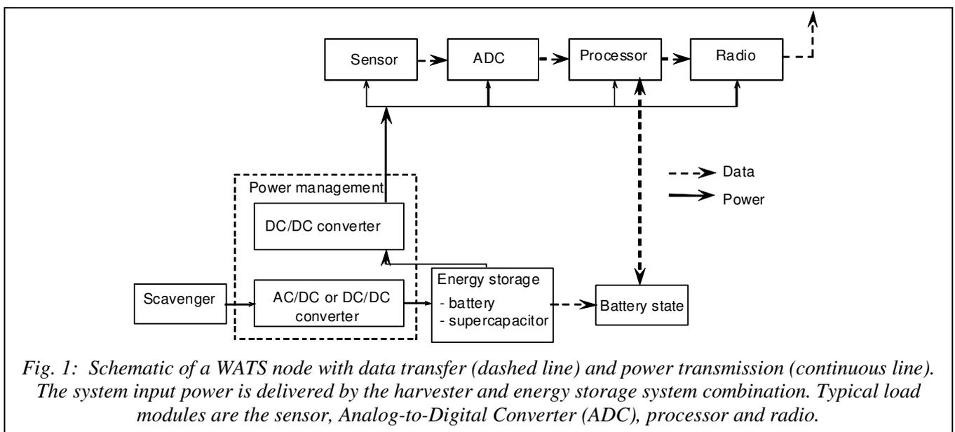
Fig. 1: Schematic of a WATS node with data transfer (dashed line) and power transmission (continuous line). The system input power is delivered by the harvester and energy storage system combination. Typical load modules are the sensor, Analog-to-Digital Converter (ADC), processor and radio.
