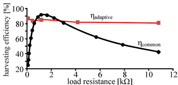
Fig. 6: Comparison of harvesting efficiencies based on the inductive generator of Fig. 5.
