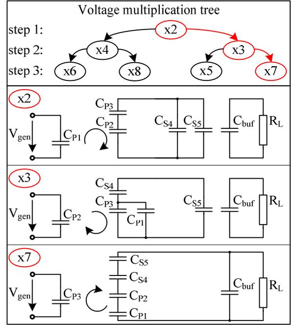
Fig. 4: Voltage conversion tree and multi-step conversion is exemplary shown for  $c_{ratio} = 7$ .
