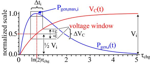
Fig. 3: Normalized capacitance charging curve  $V_C(t)$  with constant  $V_i$  is plotted. The voltage window is located around  $\frac{1}{2} V_i$  for approaching peak power transfer.
