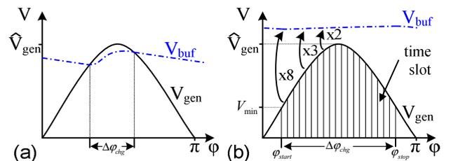
Fig. 2: Harvesting with common buffered rectifier (a) is compared to the oversampling interface (b).
