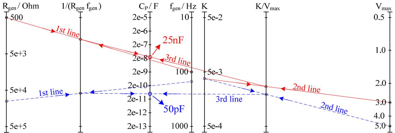
Fig. 5: Nomogram relating  $R_{gen} - f_{gen}$  to a 1<sup>st</sup> and  $K - V_{gen,oc}(V_{max})$  to a 2<sup>nd</sup> auxiliary point. Connecting both auxiliary points results in the necessary converter input capacitance  $C_{in}$  ( $K = 3.756E-03$ ). The dashed blue lines show a piezo-generator example and the red lines give an example for a typical inductive generator.
