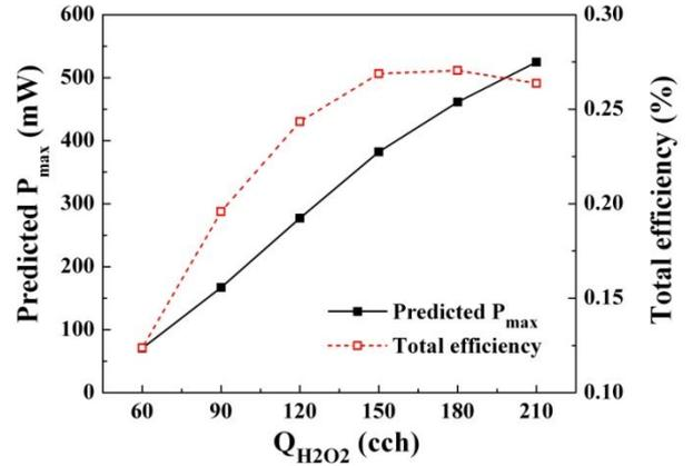
Fig. 5: Predicted  $P_{max}$  and total efficiency
