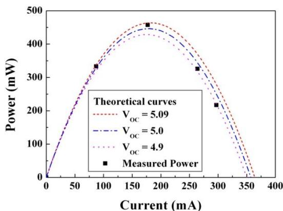
Fig.9: The predicted power curves with different  $V_{OC}$  and the measured output power with respect to the current
