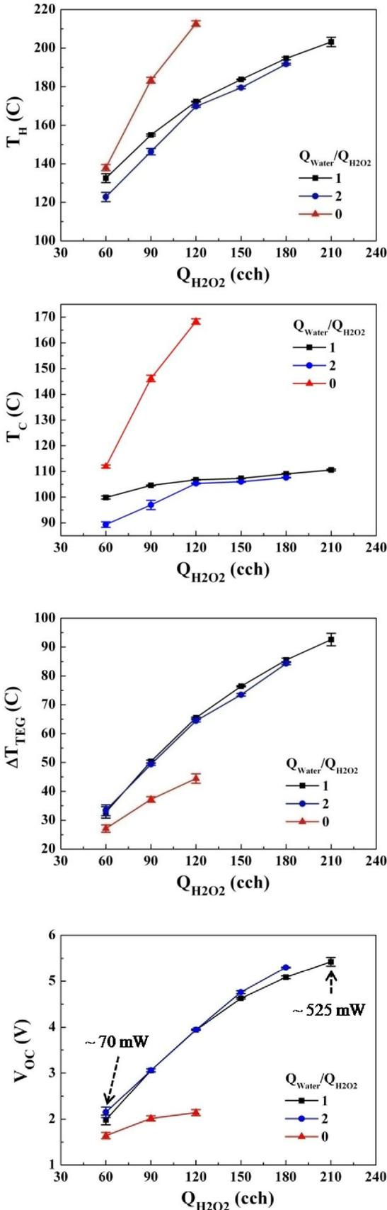
Fig. 4:  $T_H$ ,  $T_C$ , temperature differences across the TE module and the open circuit voltages with respect to the  $H_2O_2$  flow rates
