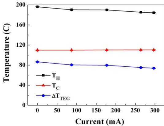
Fig. 8:  $T_H$ ,  $T_C$  and  $\Delta T_{TEG}$  with respect to the current
