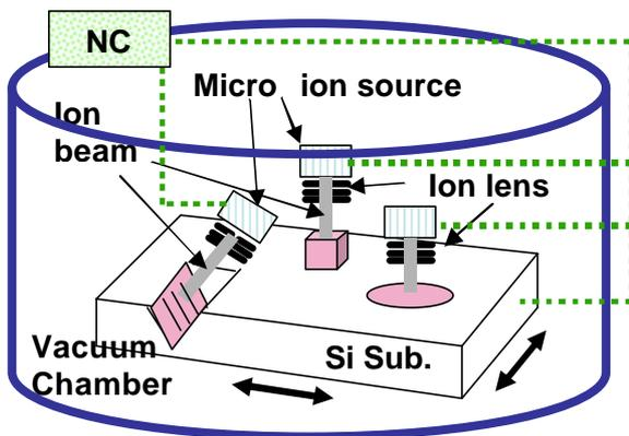
Fig.4: An example of programmable sequence process by using micro-machined micro ion source units to reduce power consumption of manufacturing
