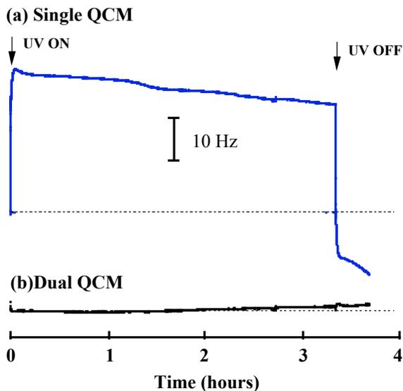
Fig. 2: An example of the correction of environmental influences on the resonant frequency by using the referenced QCM. (a) Frequency response of a single QCM. (b) Frequency response of a dual QCM. Irradiation power of UV is about 6.5 mW/cm<sup>2</sup>.
