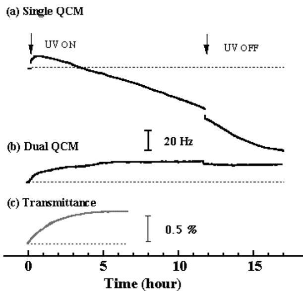
Fig. 4: Measured photo-catalytic reactions by using miniaturized QCM array [7]. The MB dye was spin-coated on the  $\text{TiO}_2$  film.
