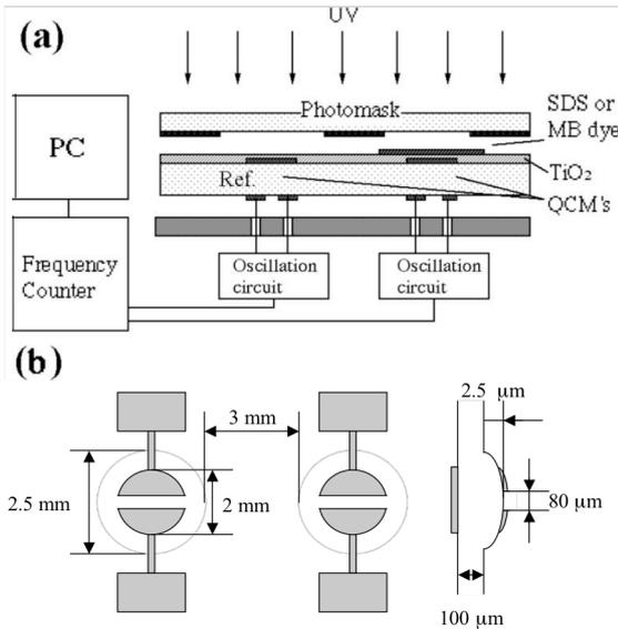
Fig. 1: The experimental set-up for the evaluation of photo-catalytic reactions (a) and the electrode configuration of dual QCM (b).
