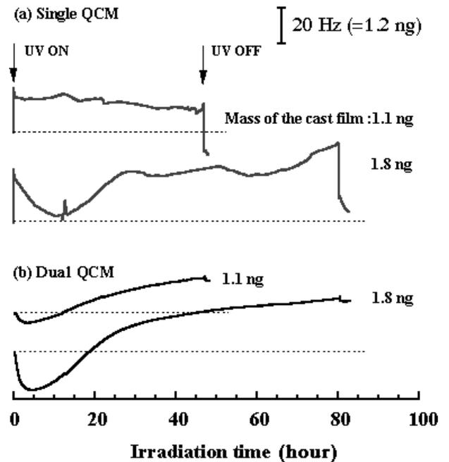
Fig. 6: Measured photo-catalytic reactions of a cast MB dye film on the  $\text{TiO}_2$  thin film by using miniaturized QCM array. (a) The frequency changes measured by single QCM. (b) The frequency changes measured by dual QCM.
