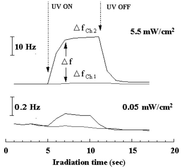
Fig.3: Frequency responses under the UV irradiation.
