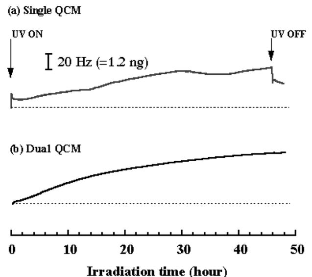
Fig. 7: Measured photo-catalytic reactions of a cast SDS film under the UV irradiation by using miniaturized QCM array. (a) The frequency change measured by single QCM. (b) The frequency change measured by dual QCM.
