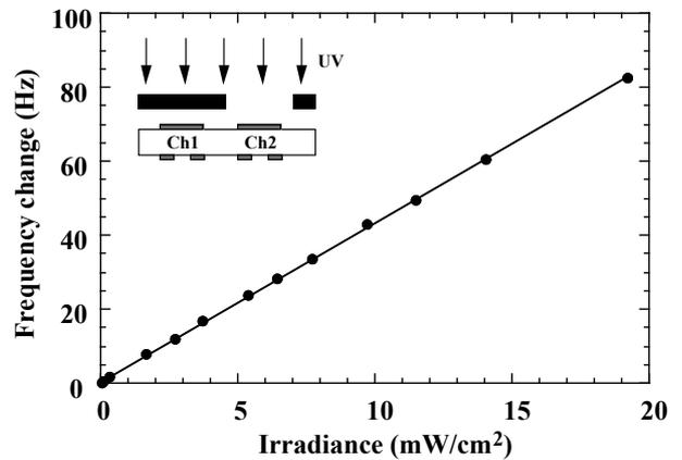
Fig. 4: Frequency changes against the intensity of UV irradiance. The diameter of the pinhole is 3 mm and that of the QCM is 2 mm.
