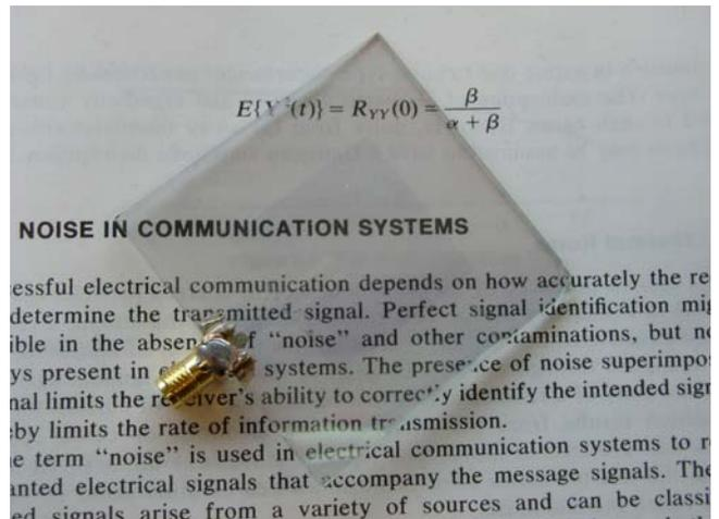
Figure 3: Example of an optically transparent (microstrip patch) antenna, realized by ITO on glass.
