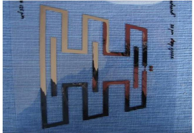
Figure 2: Three elements series array of re-entrant folded dipole antennas fabricated on PET foil.
