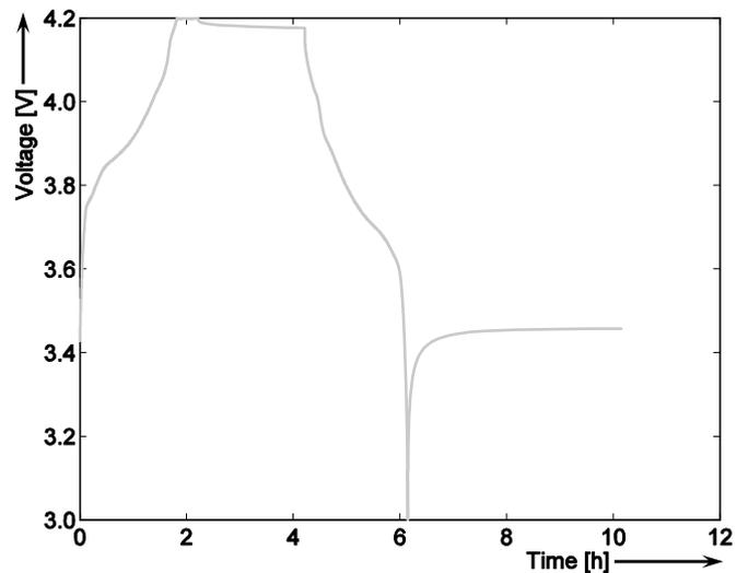
Figure 5: The voltage from the first activation cycle for the Li-ion battery as function of the experiment time in hours. The battery has been charged by means of the CCCV charging mode by limiting the (dis)charging voltage and current. In this case, voltage levels of 3.00 - 4.2 V, respectively, have been considered.
