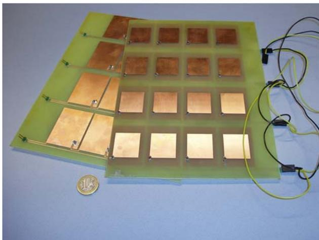
Figure 6: 2.45GHz microstrip rectenna boards, back and front views. Every row of four elements are connected in series. These four rows may be combined in parallel or series connection. For the experiment, we have used two rows only, connected in series
