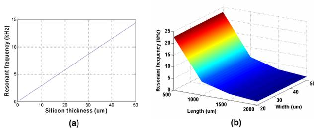
Fig. 3: Resonant frequency with respect to (a) the silicon thickness for a 50- $\mu$ m wide and 2000- $\mu$ m long cantilever, (b) the cantilever width and length for a fixed silicon layer of 5  $\mu$ m.
