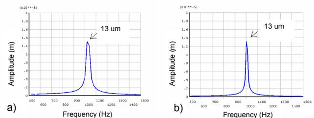
Fig. 5: Harmonic responses of PZT cantilevers (a) without a mass, (b) with a mass.
