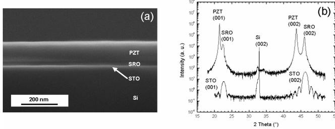
Fig. 1: (a) Cross-sectional SEM image of epitaxial PZT/SRO/STO thin films grown on a Si (100) substrate, (b) Theta-2theta diffraction scan.
