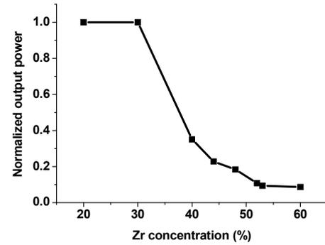
Fig. 2: Normalized output power as the function of Zr concentration based on parameters in [7].
