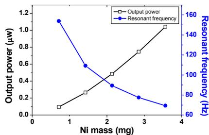
Fig. 6: Output power and resonant frequency as a function of Ni mass.
