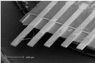
Fig. 7: SEM image of epitaxial PZT cantilever array.
