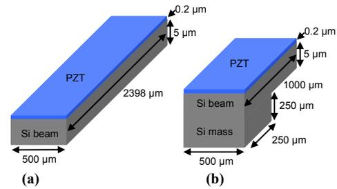
Fig. 4: Comparison of two PZT cantilevers (a) without a Si proof mass, (b) with a Si proof mass.
