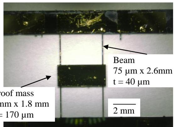
Fig. 7: Picture of the top electrode
