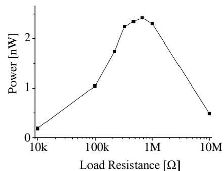
Fig. 12: The relationship between load resistance and the output power.
