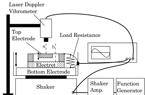
Fig. 8: Schematic of the experimental setup
