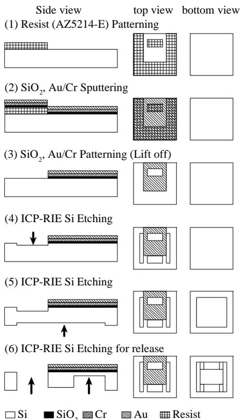
Fig. 6: Fabrication chart of the top electrode.
