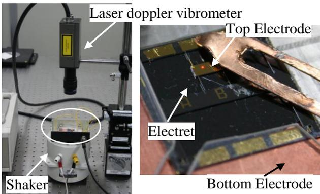
Fig. 9: Picture of the experimental setup
