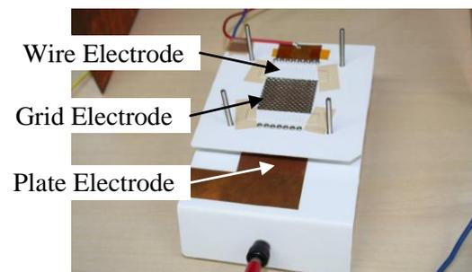
Fig. 4: Schematic and picture of corona charging system.
