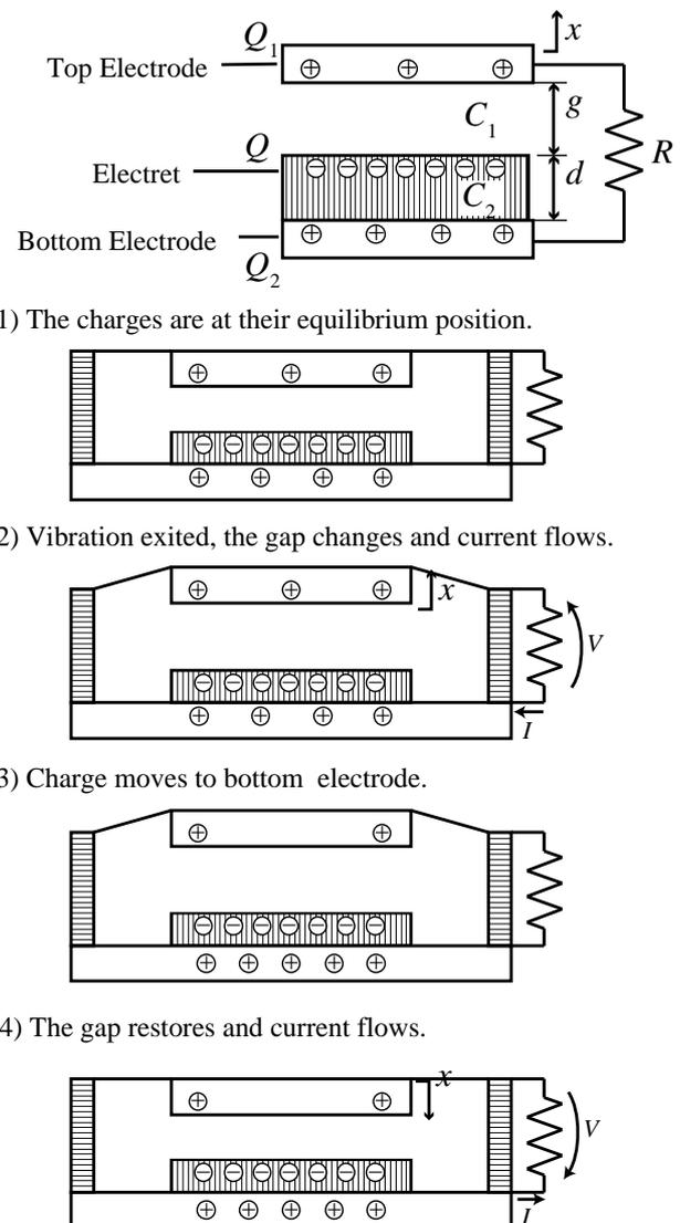
Fig. 1: The model of the generator presented in this work
