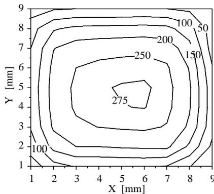
Fig. 5: Distribution of the surface potential of electret (unit: Volt)
