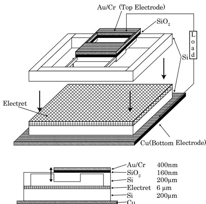
Fig. 2: Schematic of the prototype generator
