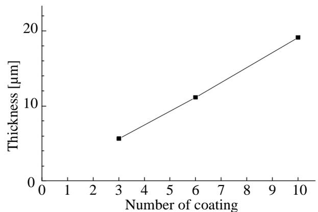
Fig. 3: Relationship between number of spincoating and the thickness of CYTOP film.
