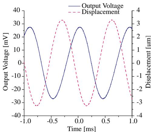
Fig. 10: The waveform of the output and the relative displacement of the top electrode.
