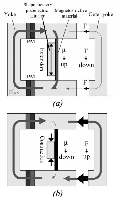
Fig. 2: (a) Extension and (b) contraction conditions of the composite model.
