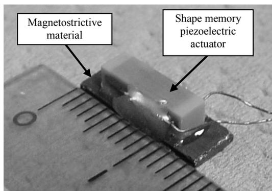
Fig. 3: A magnetostrictive-shape memory piezoelectric actuator composite.
