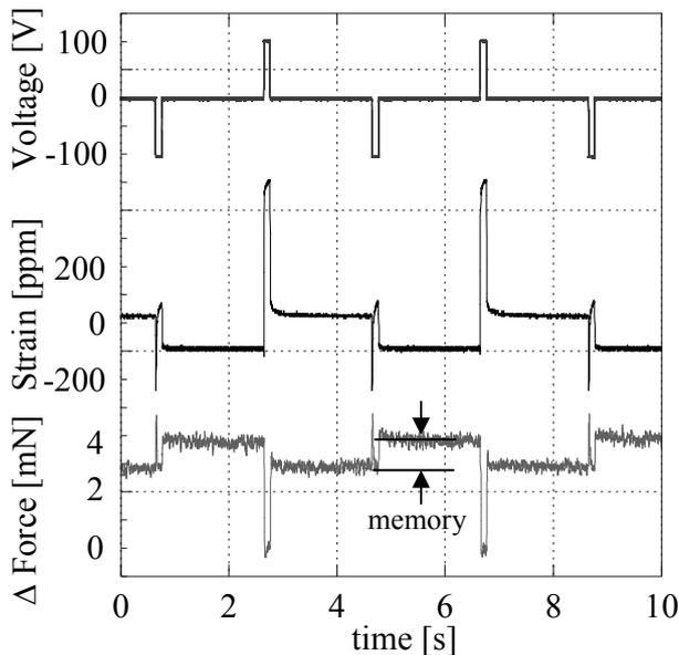
Fig. 6: Change in the piezoelectric strain and the magnetic force driven using a pulsed voltage.
