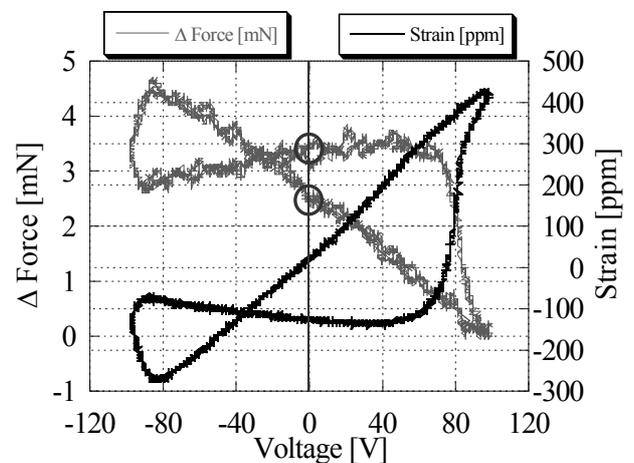
Fig. 5: Relationship between piezoelectric strain and the variation in  $\Delta$  Force with voltage applied
