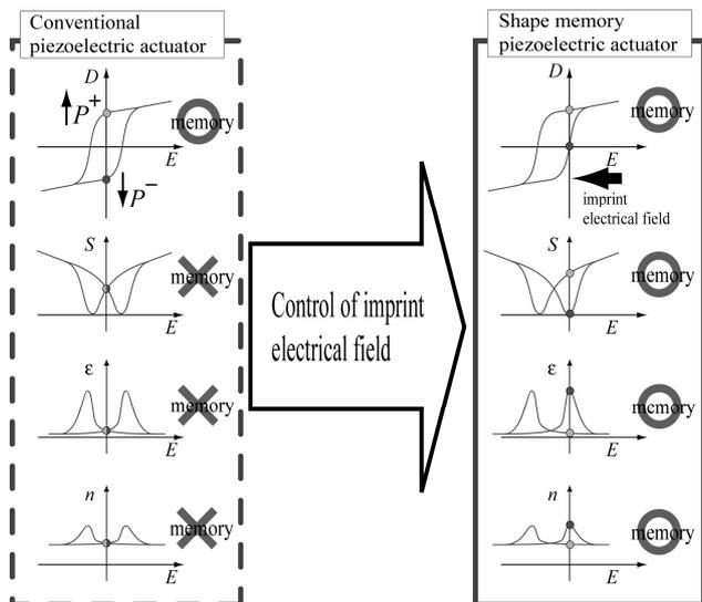
Fig. 1: Principle of the memory effect induced by control of the imprint electrical field.
