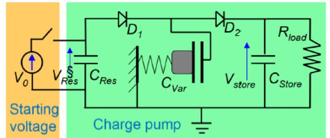
Fig. 4: The charge pump circuit
