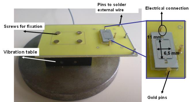
Fig. 2: Test bench with a zoom on the energy harvester
