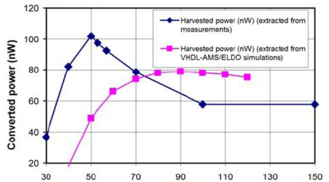
Fig. 8: Harvested power converted from the mechanical to the electrical domain in the charge-pump.
