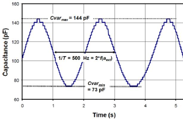
Fig. 3: Measurement of one of the transducer's capacitance variation with applied external acceleration equal to 0.1 g.
