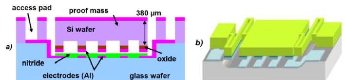
Fig. 1: Proposed energy harvester design: a) side view, b) 3d-view [1].
