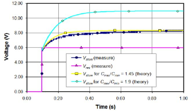
Fig. 5: Measurement and theoretical evolution with time of  $V_{res}$  and  $V_{store}$  with an infinite load after an initial pre-charge of  $V_0 = 6$  V on  $V_{res}$ .
