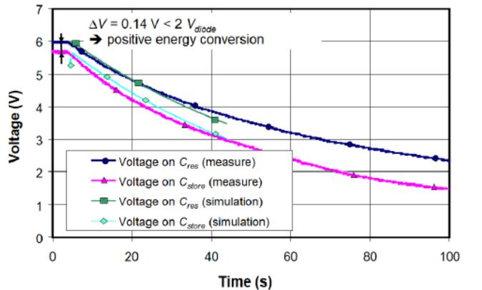
Fig. 6: Measurements and simulations of the charge-pump operation in autonomous mode on a 50 MΩ load resistance for a pre-charge of 6 V.
