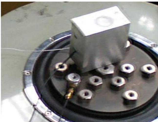
Figure 6 test setup for electrets power generator mounted on shaker
