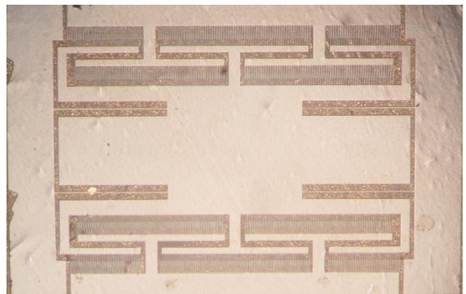
Fig. 5 Photograph of the movable structure
