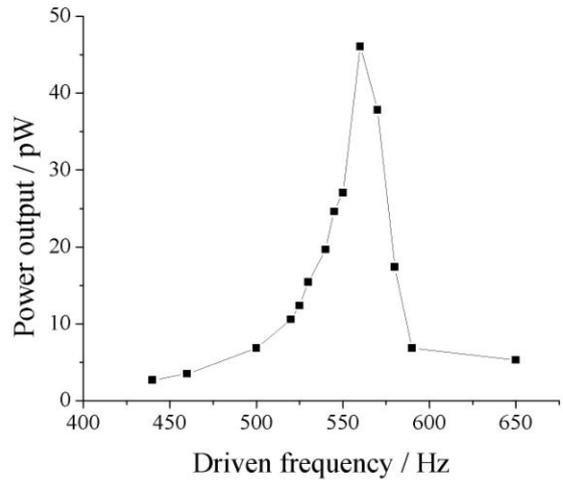
Fig. 7 Average power output at different frequencies with 1MΩ resistance
