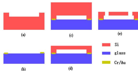
Fig. 4 The process flow for fabricating the movable structure
