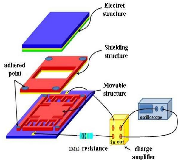
Fig. 1 Schematic graph of our new electret micro power generator
