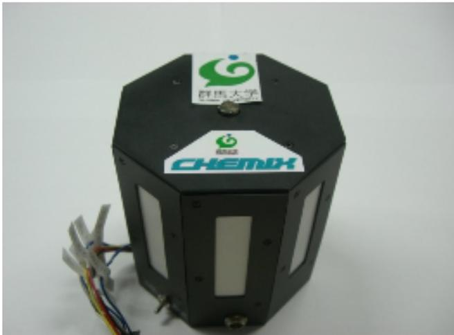
Fig.4 The prototype of passive DMFC.
