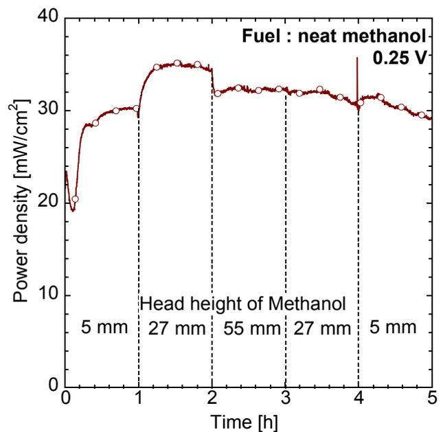
Fig.3 : Effect of methanol level on the power density profile at cell voltage of 0.25 V with neat methanol.
