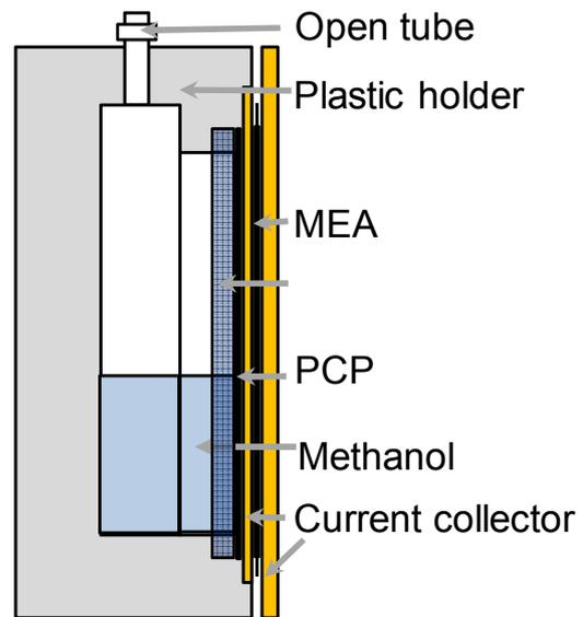
Fig.2 : Schematic diagram of experimental set-up of the single cell.
