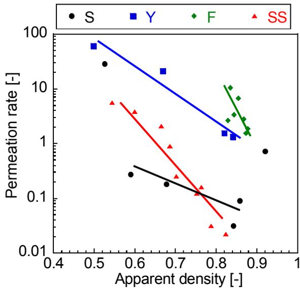
Fig.1 : Influence of the apparent density and types of PCPs on the methanol permeation rate.
