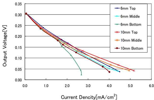
Fig. 10. Current density vs. output-voltage for each segment of the cathode.
