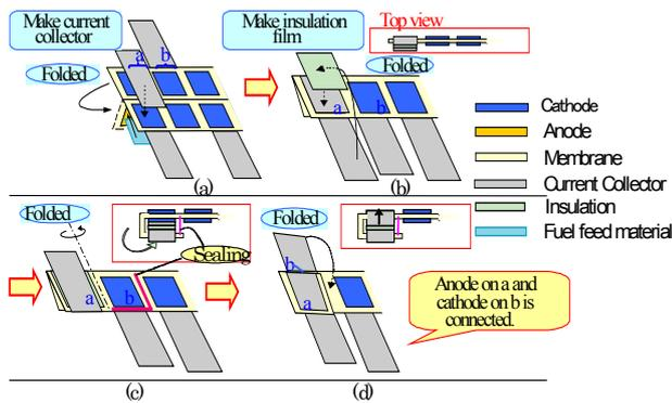
Fig. 2. Fabrication process for a zigzag-type DMFC.
