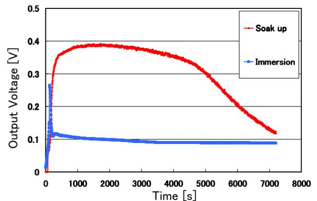
Fig.8.Operation time vs. output-voltage characteristics for soak-up and immersion fuel supply methods.
