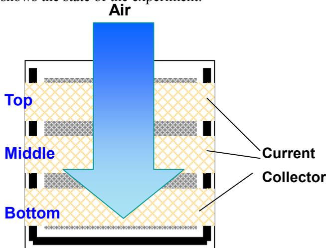
Fig. 6. Experimental set-up for air supply to the entire cathode area.
