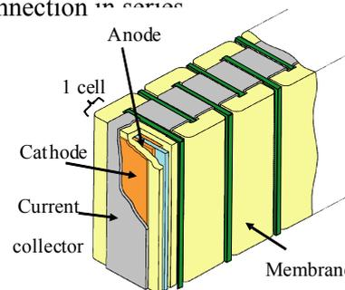
Fig. 1. Schematic diagram of a zigzag-type DMFC.
