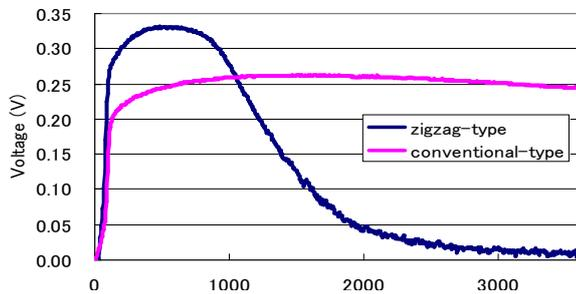
Fig. 3. Output voltage characteristics for plate-type and zigzag-type DMFCs.
