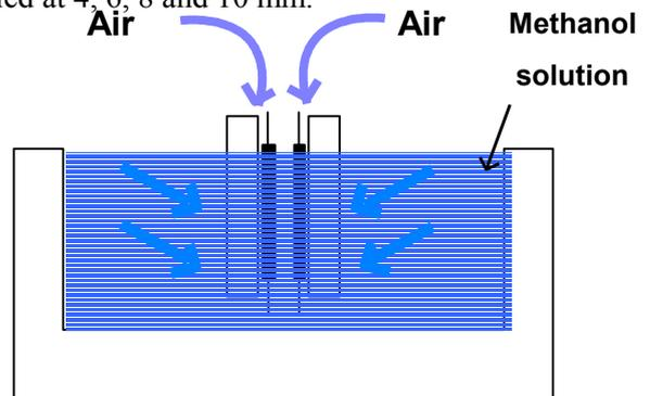
Fig. 5. Experimental set-up for the immersion fuel supply method.
