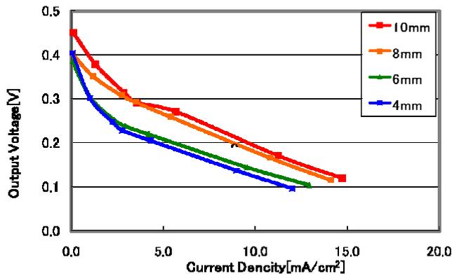
Fig.9. Current density vs. output-voltage characteristics for each cathode width.
