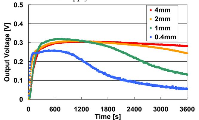
Fig. 7. Operation time vs. output-voltage characteristics for different filter paper thickness.
